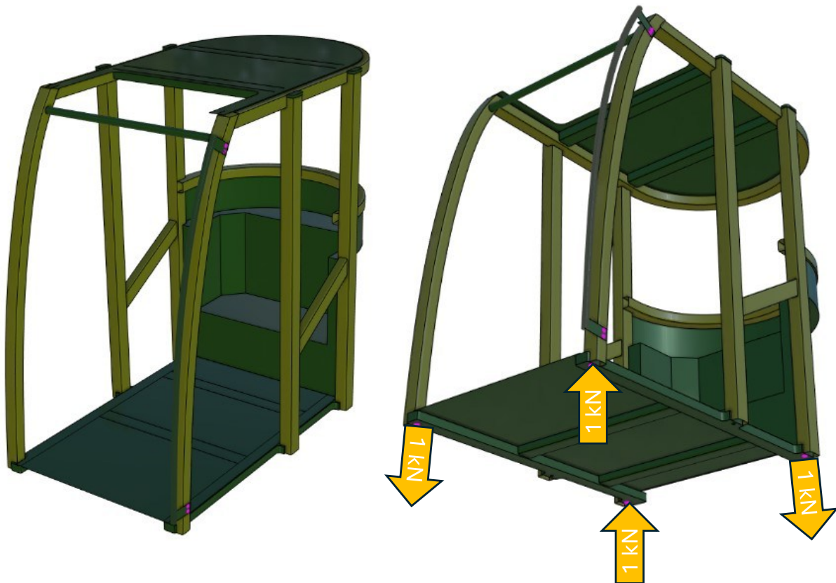
Figure 9. The left image shows the FE-model of the ROPS. The right image shows the applied loadings.
