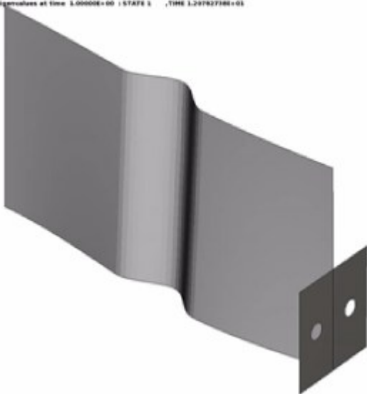
Figure 19. The lowest buckling mode shape for the panel.
