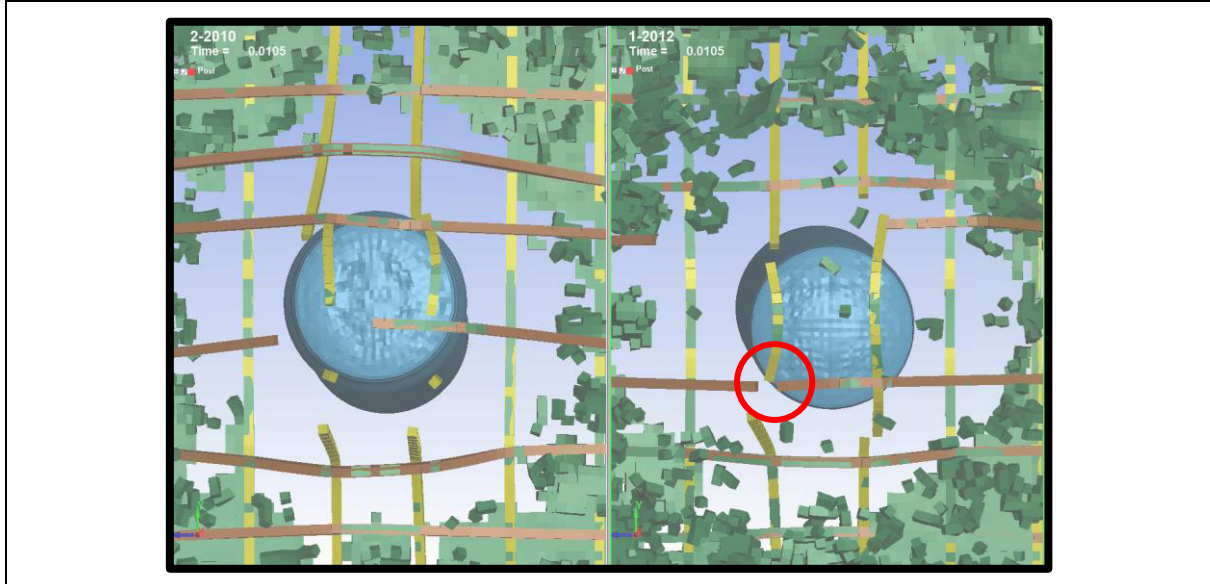
Fig.19: T=10.5\text{ms} no rebar to retain the missile for 2012 model
