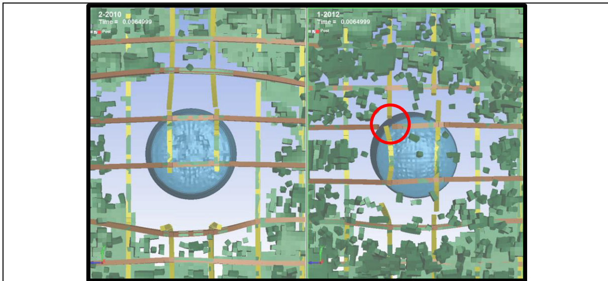
Fig.18: T=6.5\text{ms} Only one rebar remains in contact with missile for 2012 model
