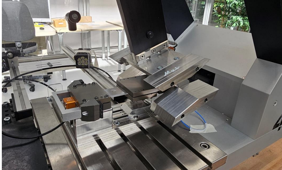
Fig.2: Test setup for dynamic shear tension tests
