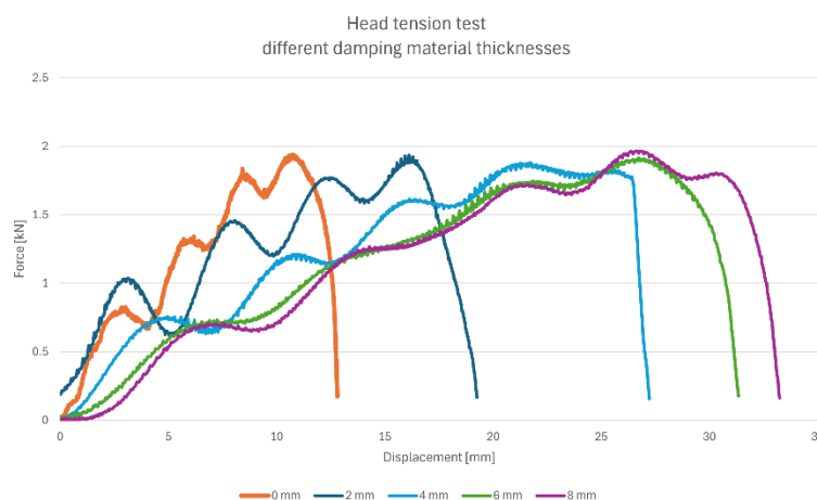
Fig.10: Head tensile test results of 1 mm thick aluminum sheet with different damping material thicknesses joined with semi-tubular self-pierce rivets
