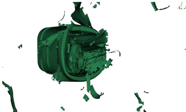
Fig.18: Final deformed shape of Tube 1A using *MAT58, showing significant elastic recovery.
