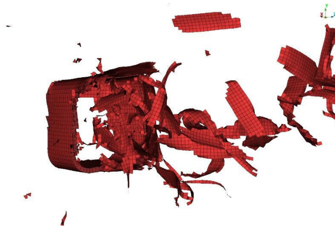
Fig.17: Final deformed shape of Tube 1A using *MAT262, showing large element elimination.
