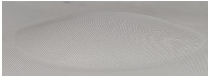
Fig.18: Permanent “plastic-like” strain after a permeability test.
