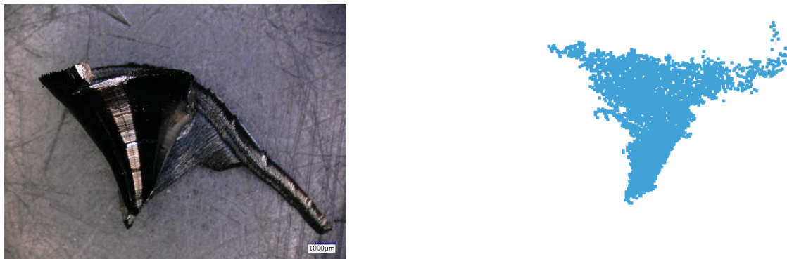
Fig.4: Chip morphology from experiment (left) and simulation (right)
