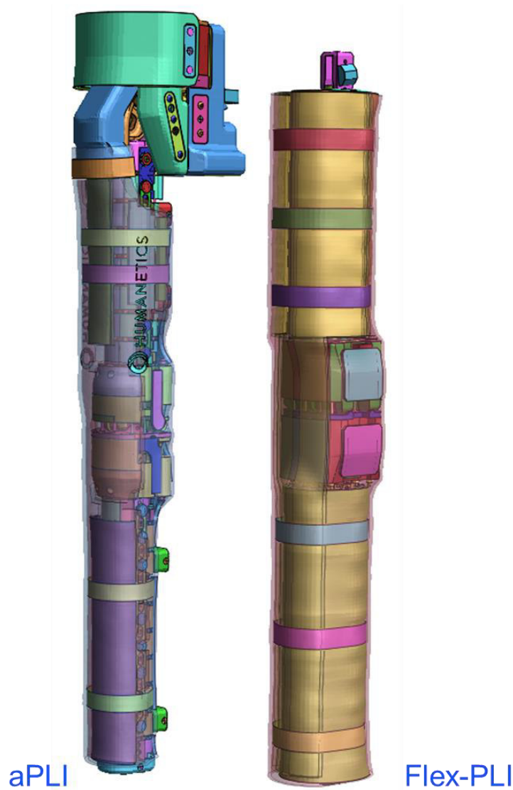
Figure 17 – View of both Humanetics aPLI (v1.2) and Flex-PLI (v1.5.1) ATD impactors, upper body mass and differing knee construction can be visualised compared to Flex PLI
