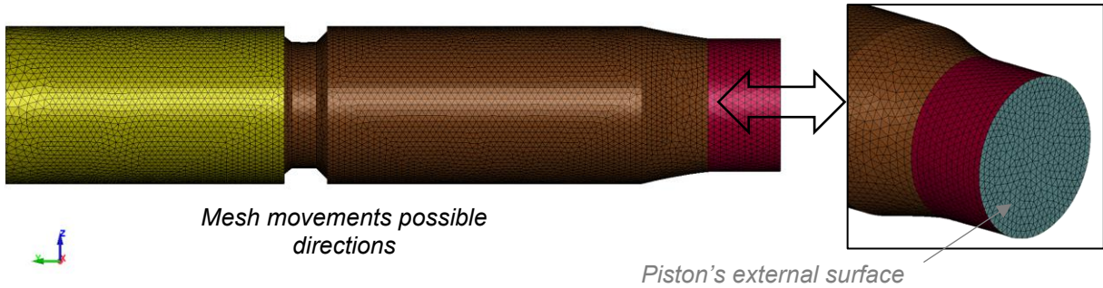
Fig.16: Piston modeling: mesh motion
