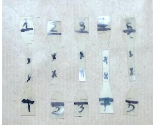
Fig.9: Fracture surface of the test specimens. Source: CARMAT
