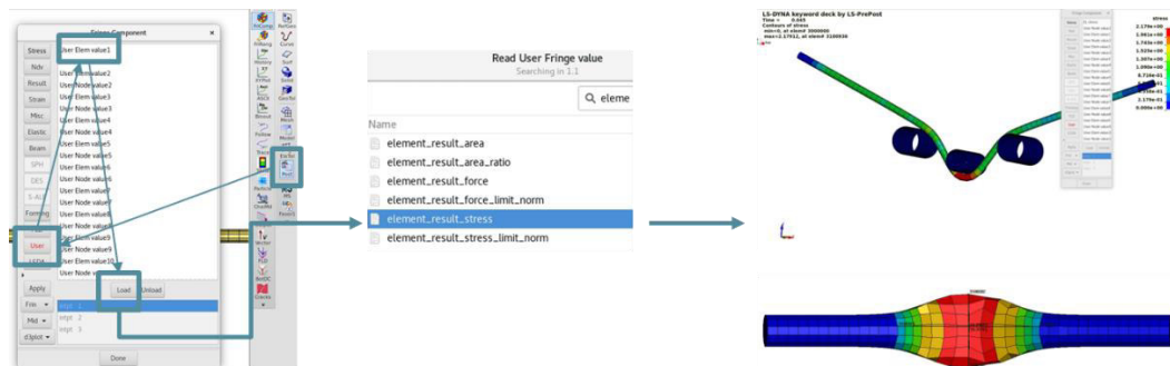
Fig. 16: User Element Result from binout to d3plot by a Python script
