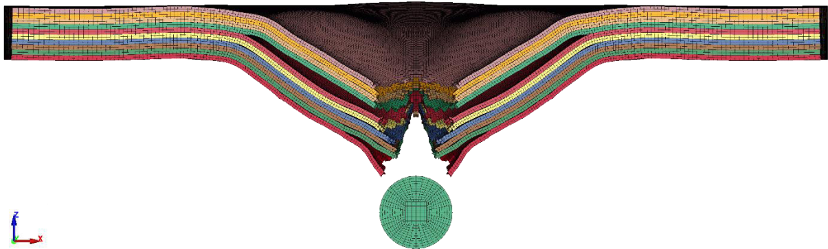
Fig.17: The simulation of Test 10 using material properties calibrated for residual velocity from LS-OPT. The simulation depicts a projectile at 66 \mu s and an initial velocity of 594 m/s with the model reflected about the YZ axis.
