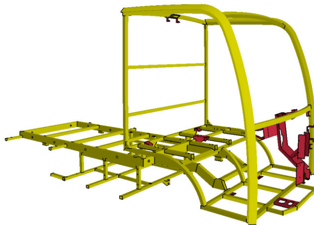
Fig.3: Material assignment plot of the BIG-e vehicle model
