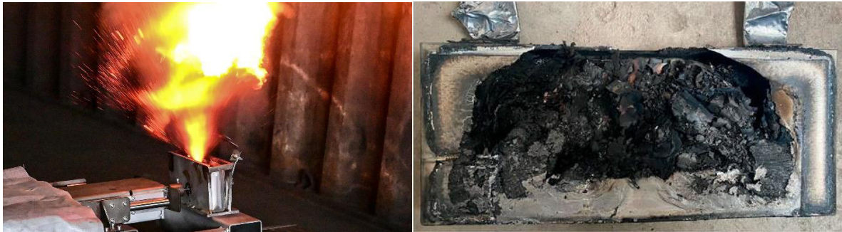
Fig 3. EV Battery Thermal Runaway testing
