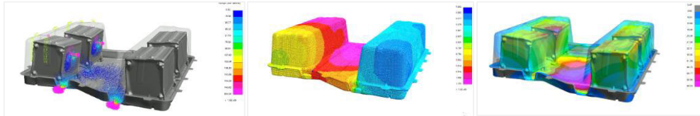
Fig 5. Flow of Gas, Temperature and Deformation Plot
