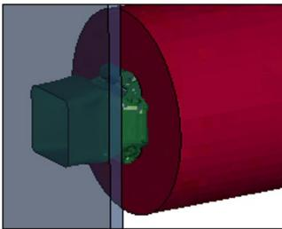
Limited creasing in crash box 3 (green) due to missing self contact
