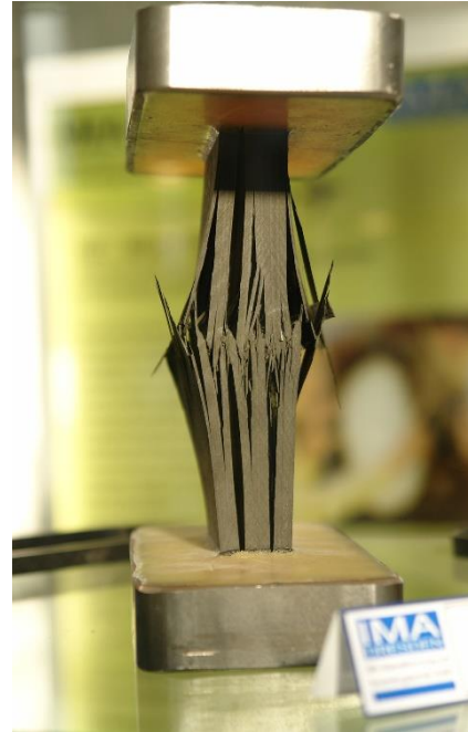
Delamination of carbon fiber-reinforced polymer under compression load. 2
