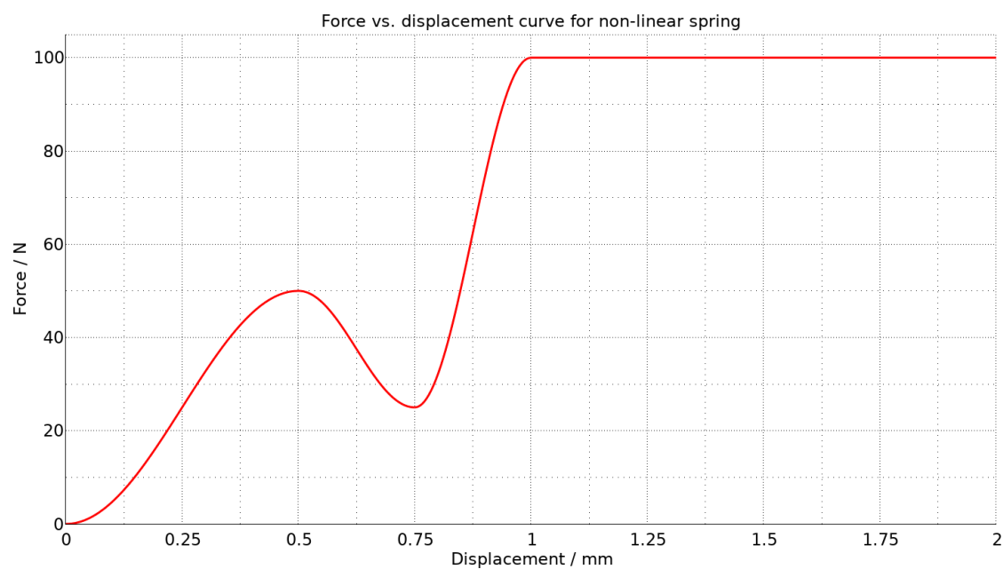
Figure 19. Non-linear force-displacement curve, input to the discrete beam material model.
