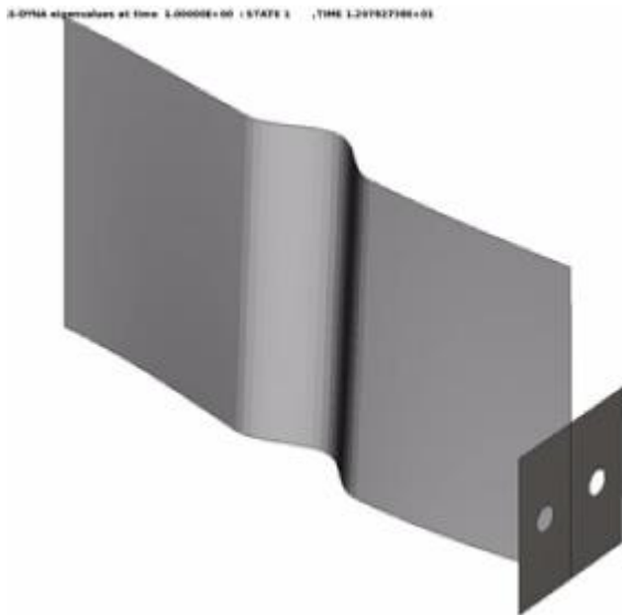
Figure 16. A panel with a bead under compression loading.
