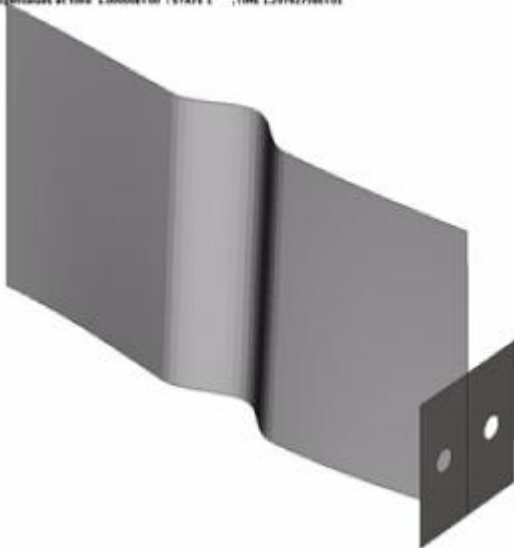
Figure 17. The lowest buckling mode shape for the panel.
