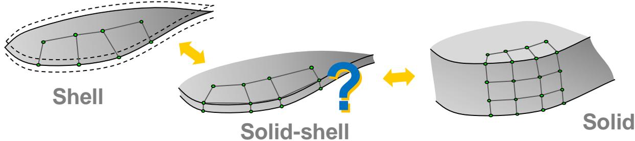
Shell elements work very well for thin structures!
