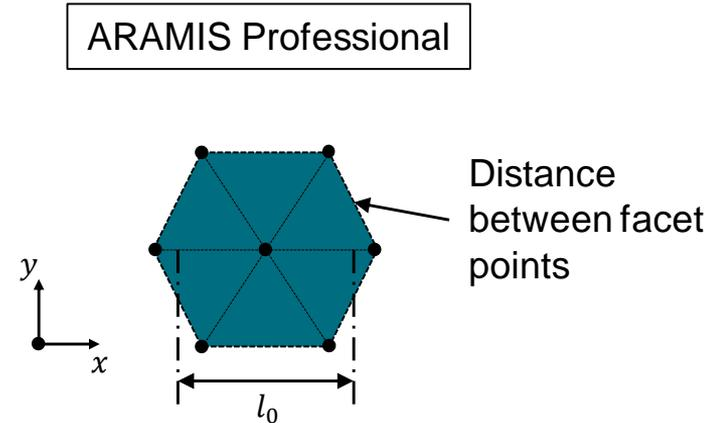
The reference length  $l_0$  in any direction is determined by the mean length of the hexagon. (0.75\*double\_facet\_point\_distance)
