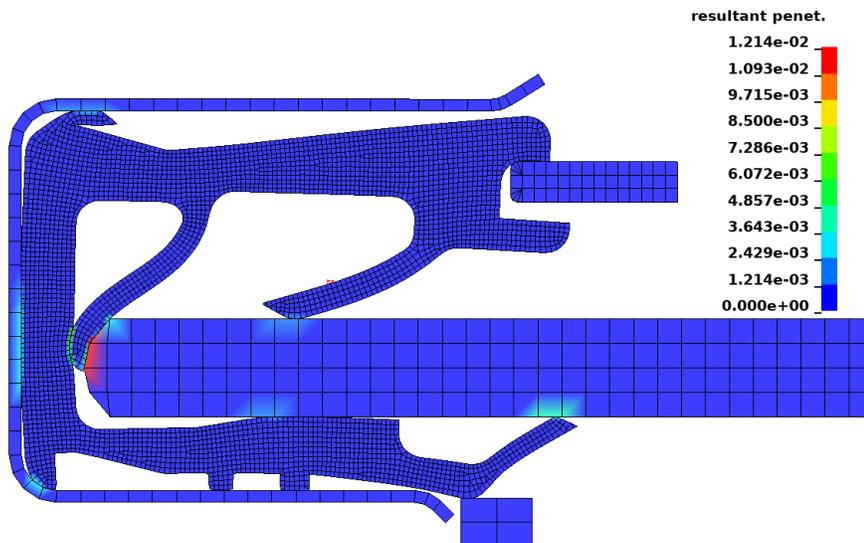
*Comment: Fringe plot of contact penetration in the MORTAR-contact.*
