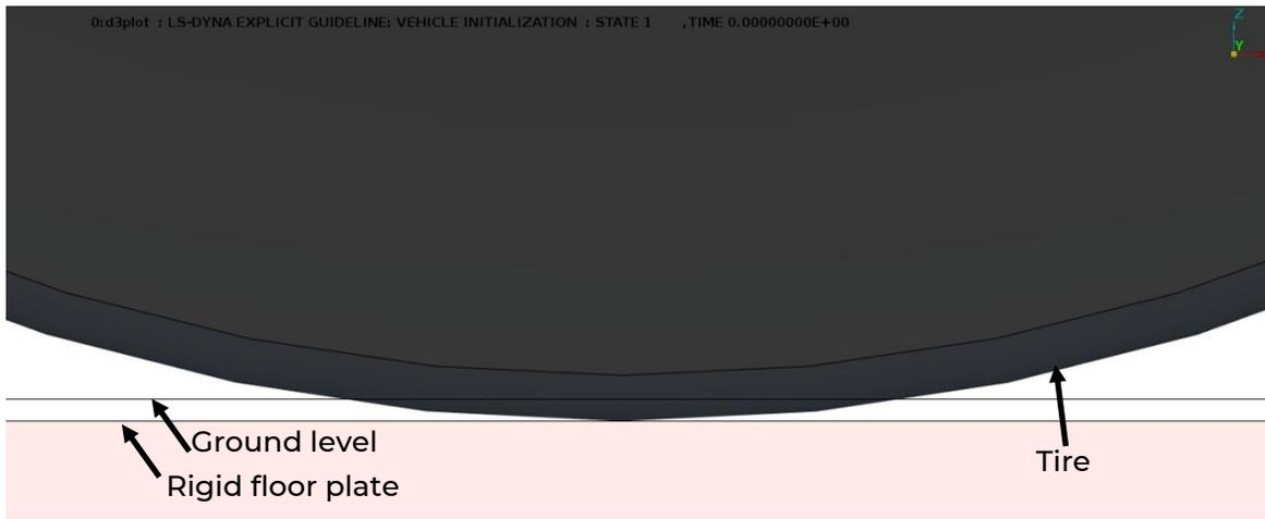
*Comment: The initial position of the vehicle/tire showing ground level and floor plate.*
