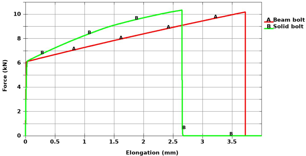
Comment: Tension test results for the beam bolt and the solid bolt, respectively.
