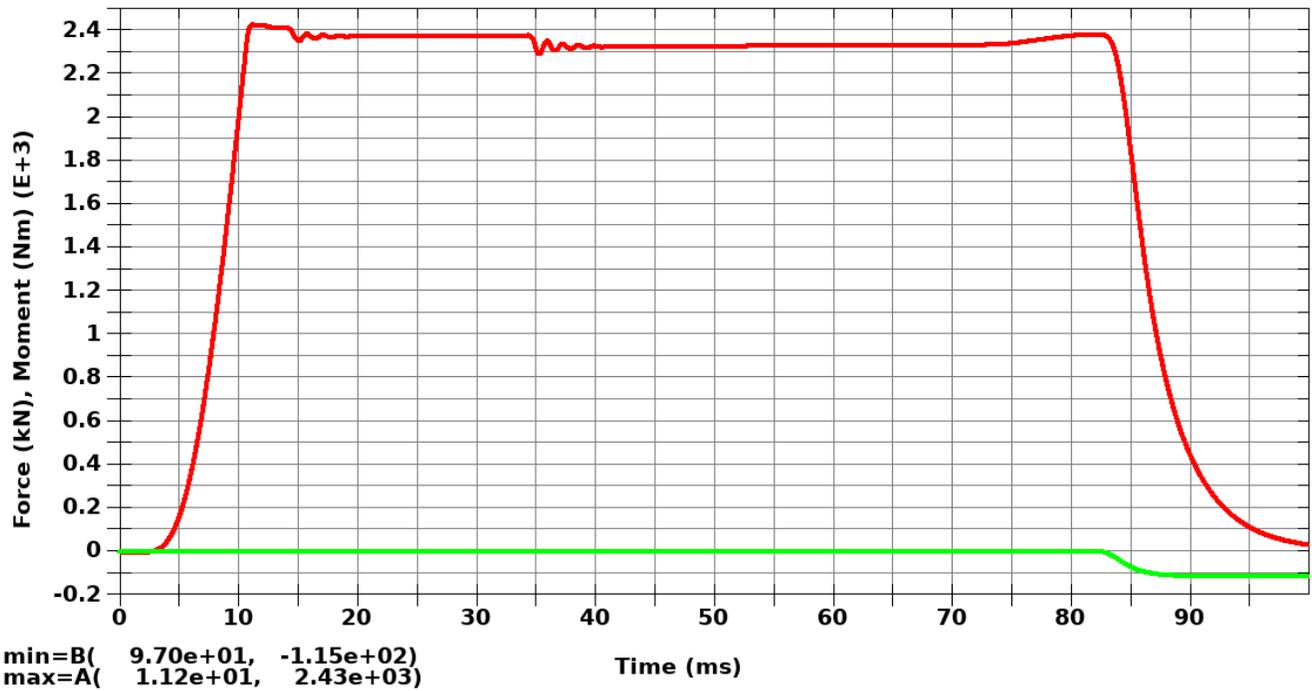
Comment: Transmission torque (red curve) and transmission axial force (green curve). BW 1000Hz filter applied.
