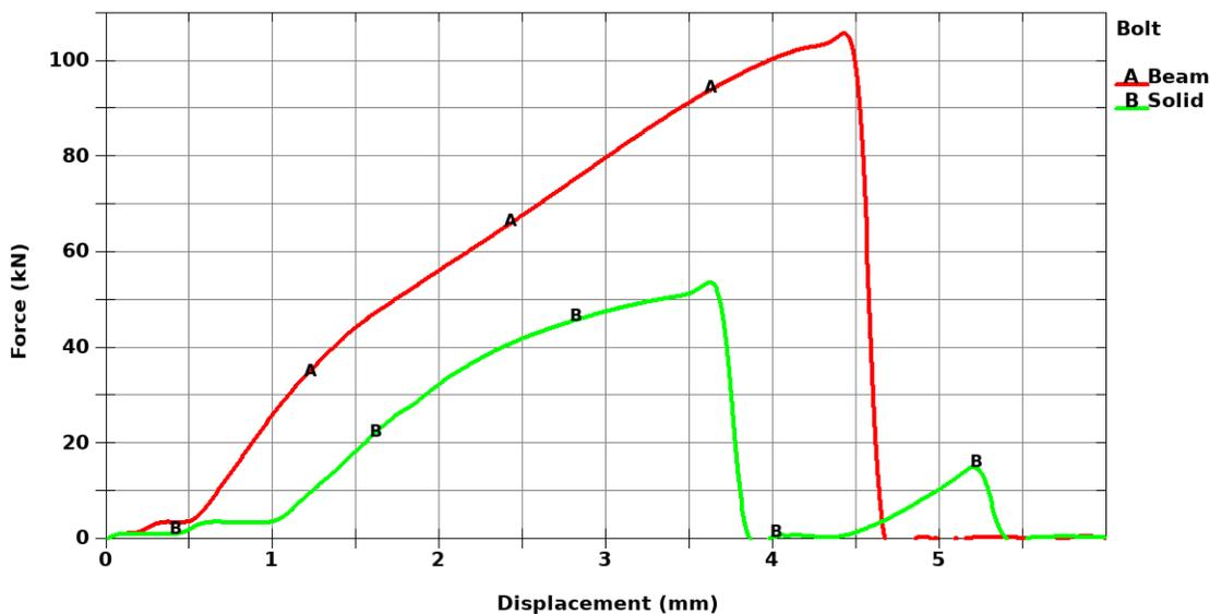
*Comment: Ultimate load (x-force) for the loading case where the connections are pulled apart. Beam element variant in red and solid element variant in green. BW 3000Hz filter applied.*
