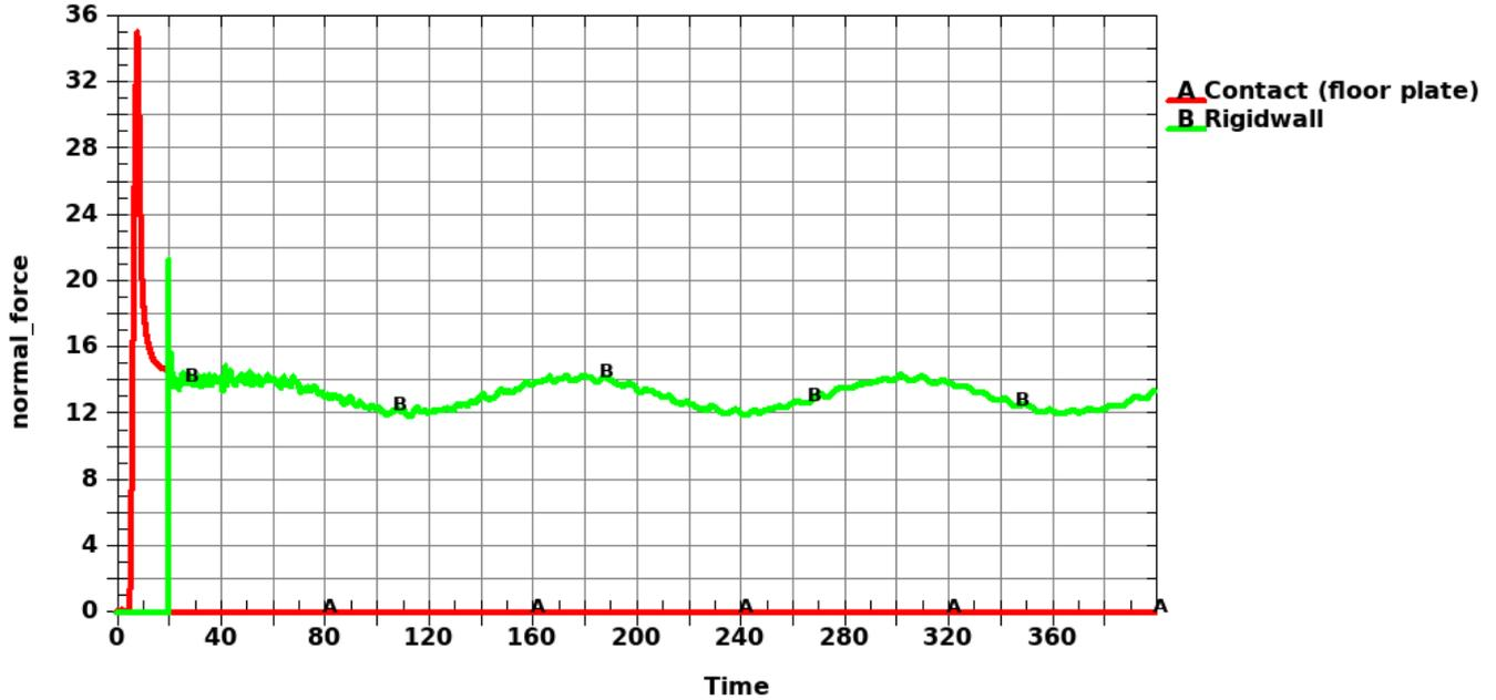
*Comment: A “steady state” analysis (no velocity applied) to check static equilibrium. A switch of any contact or rigid wall will introduce noise, see spike in green curve.*
