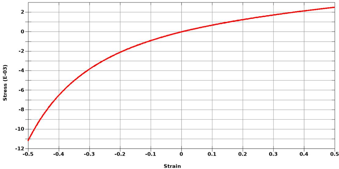
*Comment: The stress-strain curve was produced through axial tension and compression of a one-element model.*
