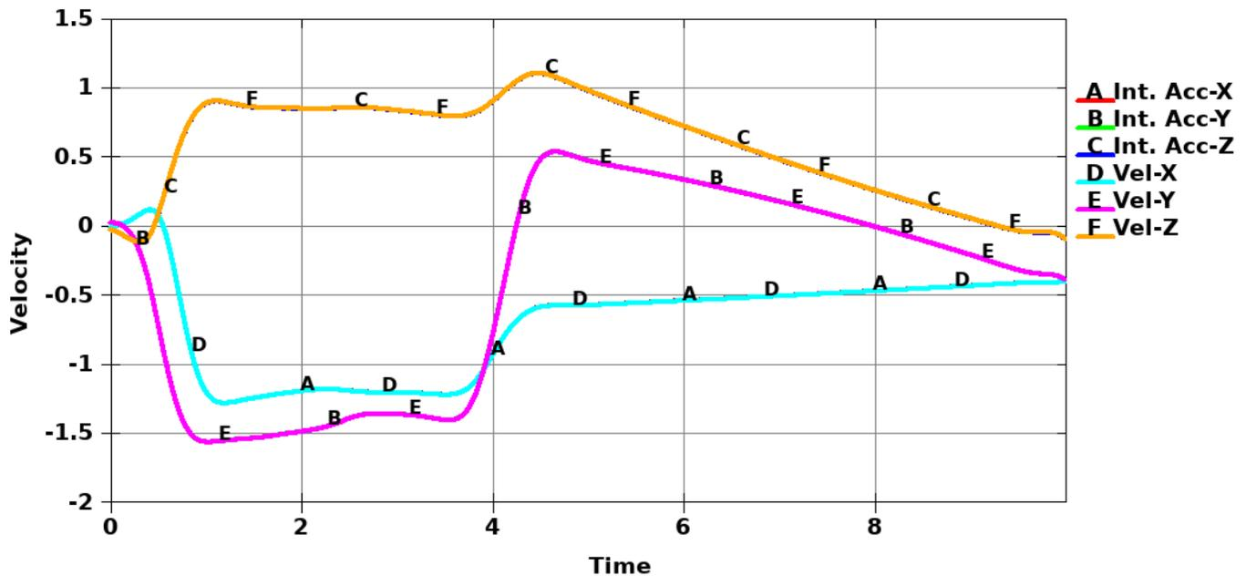
*Comment: The integrated accelerations and the velocities match (nodout, global node). A Butterworth filter with a cut-off frequency 1000 Hz is applied.*
