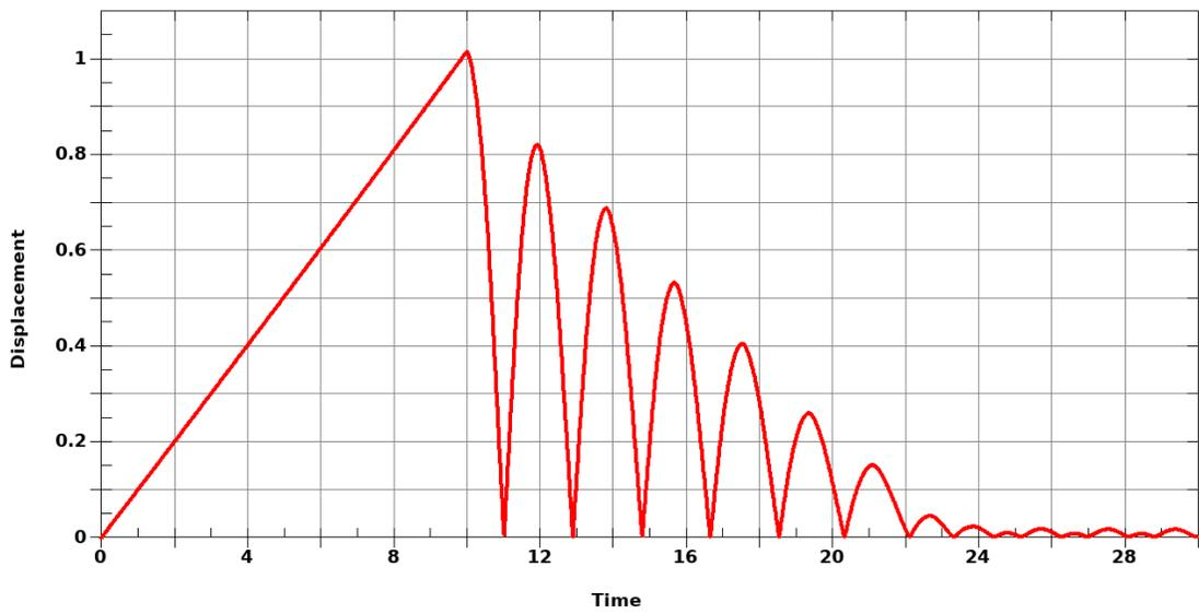
*Comment: The damping curve was produced by simulating the damped oscillations of a solid element beam.*
