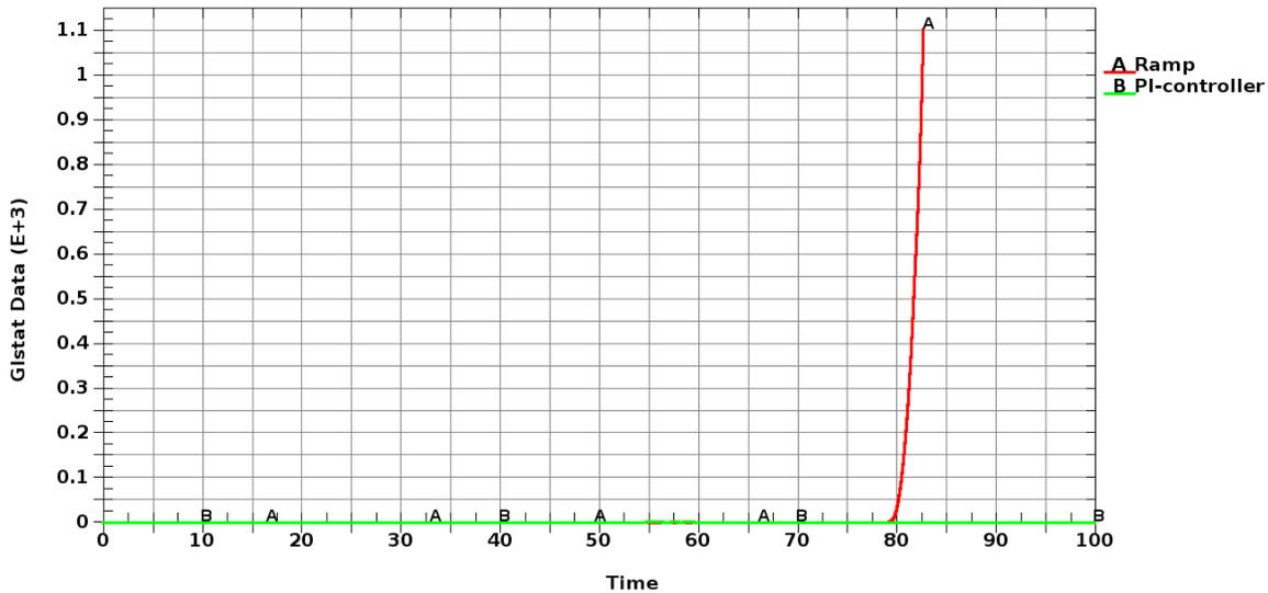
Comment: Kinetic energy with a ramp load (red curve) and with a PI-controller (green curve).
