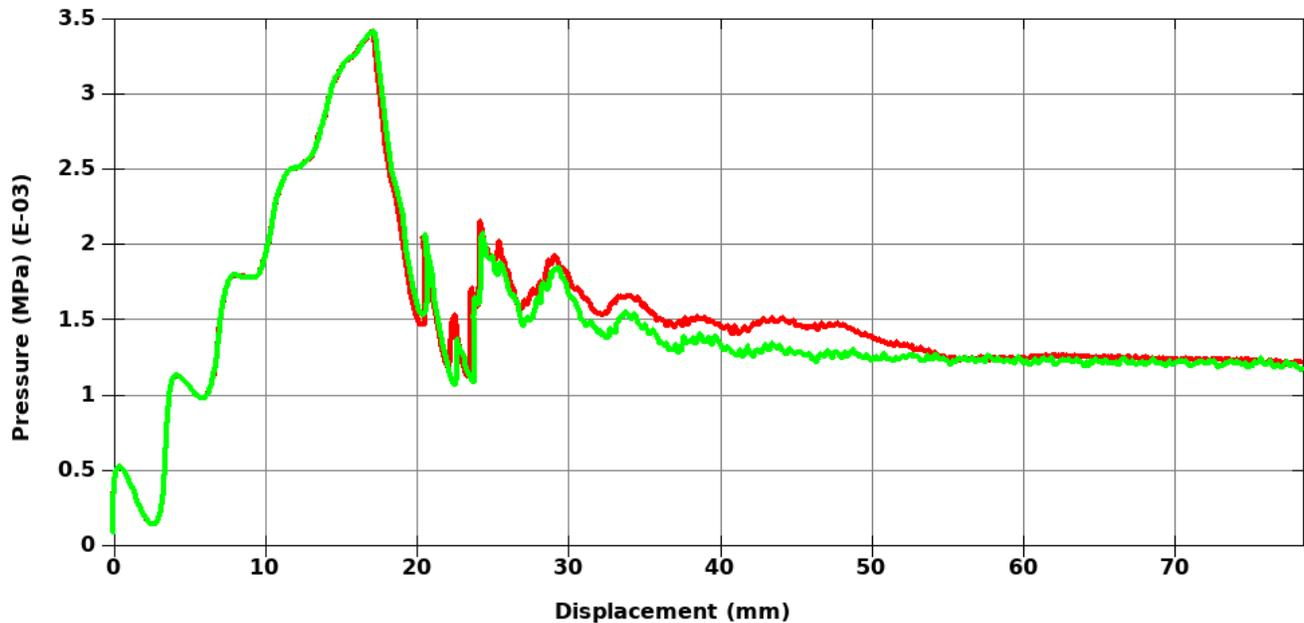
Comment: Pressure vs. displacement. Conventional mass scaling (red curve) and selective mass scaling (green curve).
