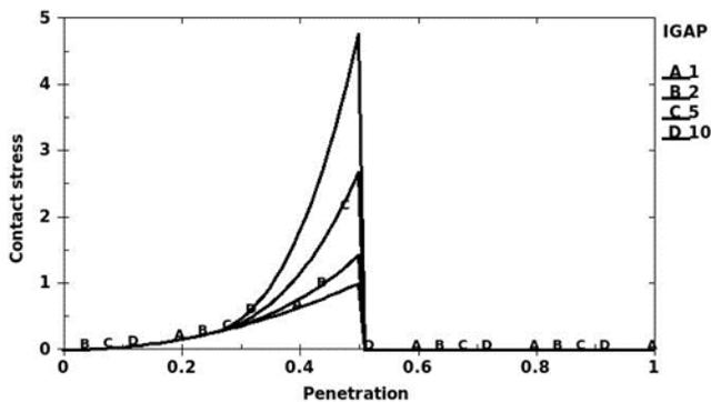
For tied contacts using penalty formulation (Option 4: OFFSET/BEAM\_OFFSET) it has been observed that reducing the penalty stiffness, e.g. SFSA=SFSB=0.1, can increase the numerical stability. This type of stability issues may be observed through strange contact energies in sleout/glstat.
