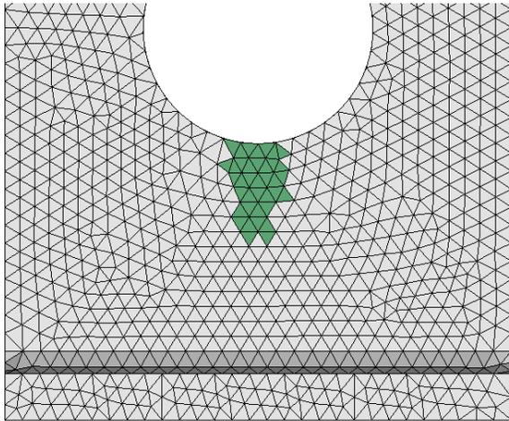
Comment: The weld line is given a separate PID by Envyo (green in figure).
