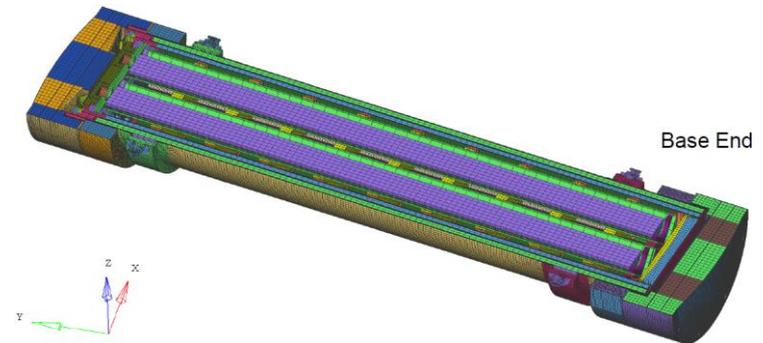
FE model utilises half symmetry of M4/12 package
