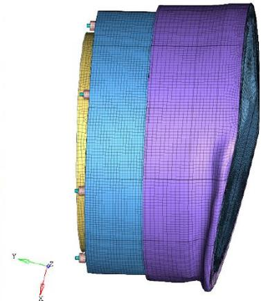
Test vs FEA – Measure of Impact deformations
