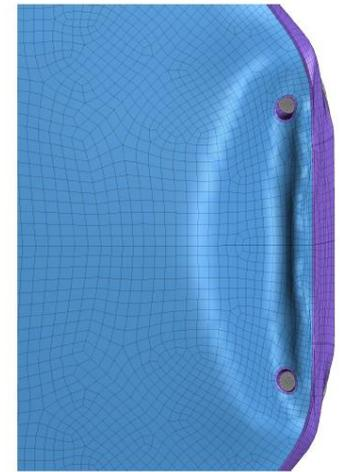
Test vs FEA – Measure of Impact deformations
