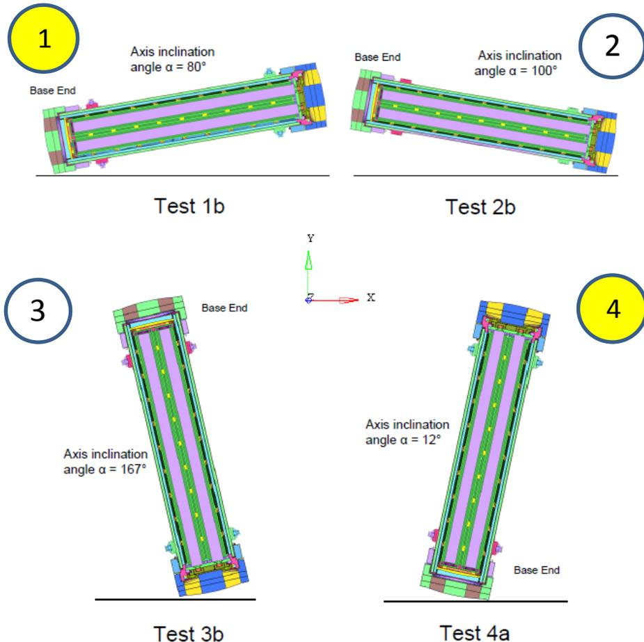
**Drop orientations in impact analysis with varying angles for base and lid end impacts**
