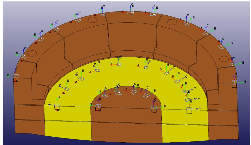
**Material directions of wood in Shock Absorber: LCC
