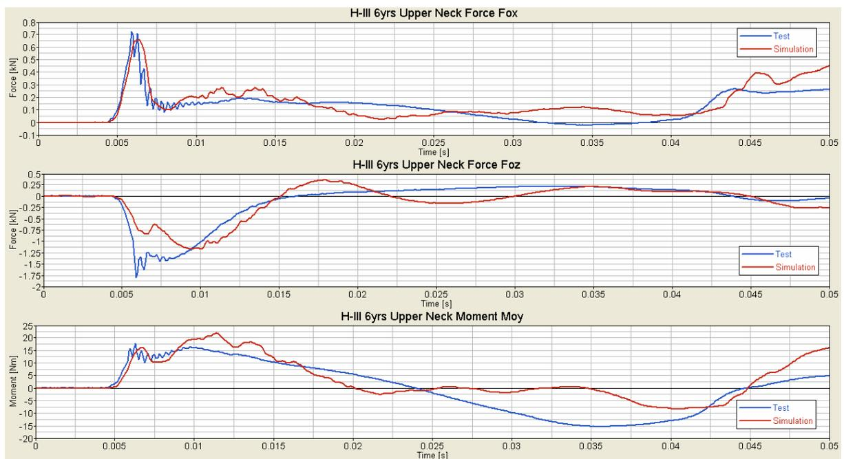
Figure 14: Comparison force simulation - test
