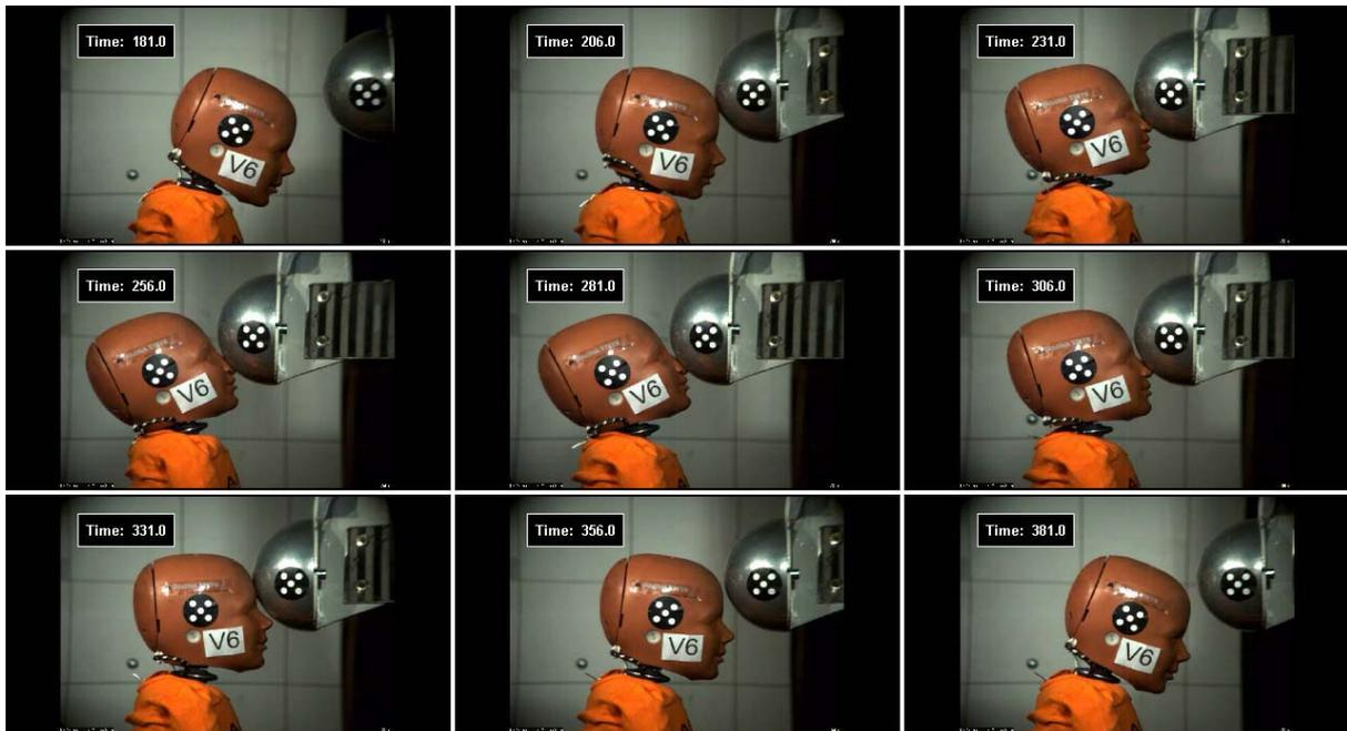
Figure 5: Test pendulum impact with 3yrs child dummy
