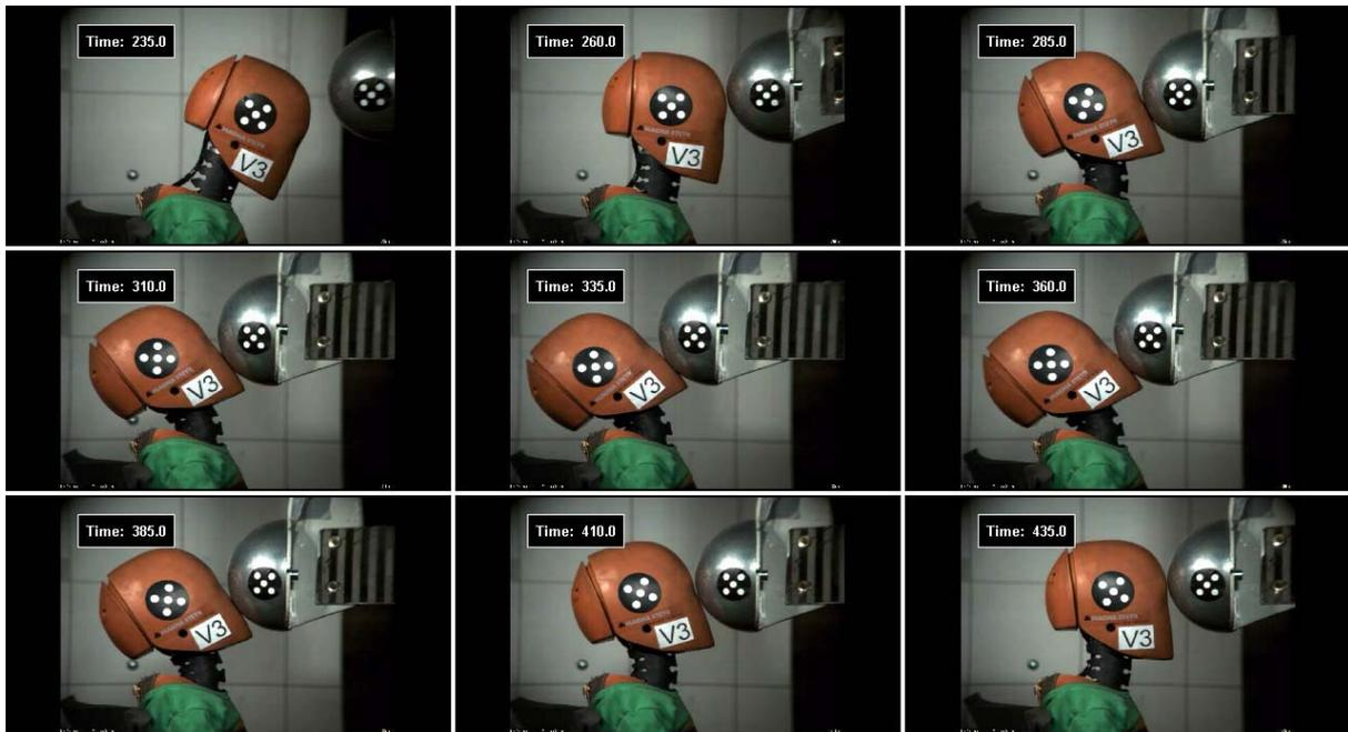
Figure 10: Test pendulum impact with 6yrs child dummy
