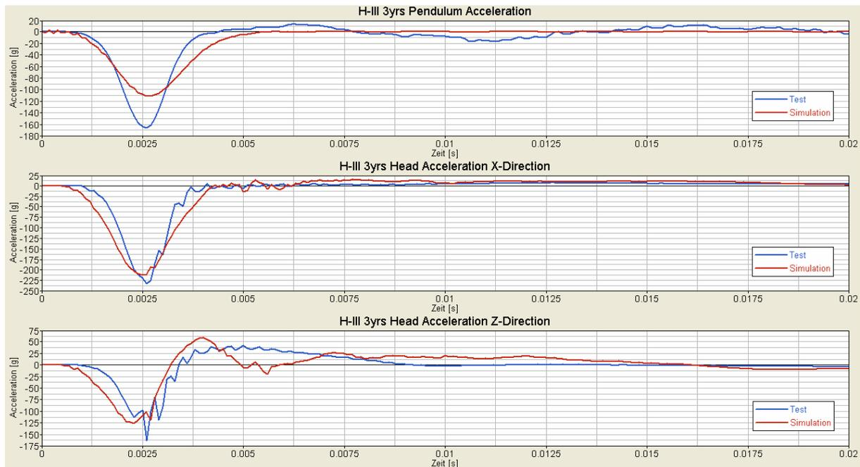
Figure 8: Comparison acceleration simulation - test
