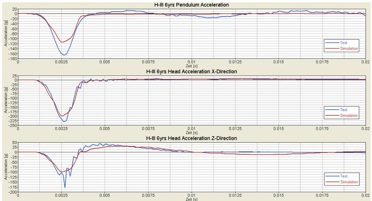
Figure 13: Comparison acceleration simulation - test
