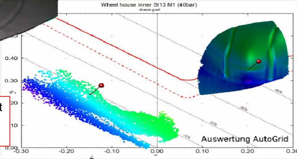
The critical area, in which the part fails, cannot be predicted using the standard FLC
