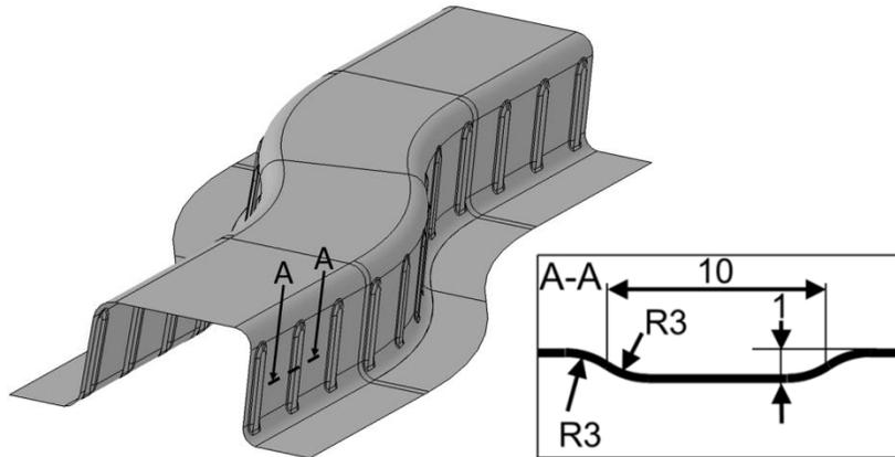
Tool geometry for restriking operation
