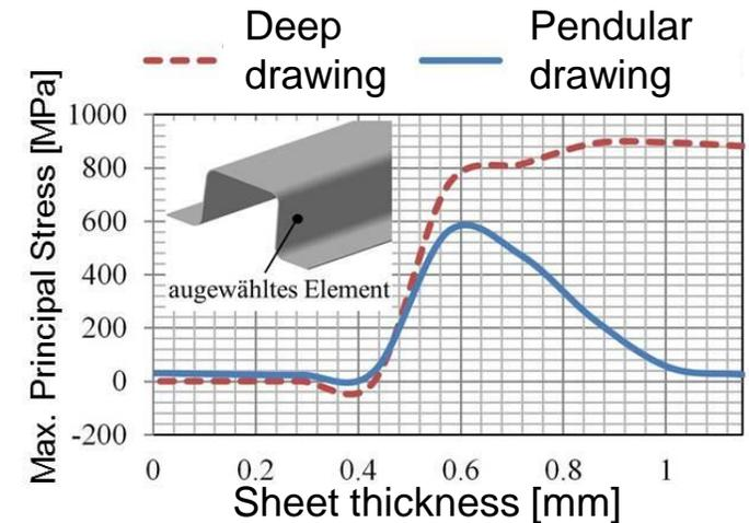
Stress distribution in sheet thickness by deep drawing and Pendular drawing for a selected finite element
