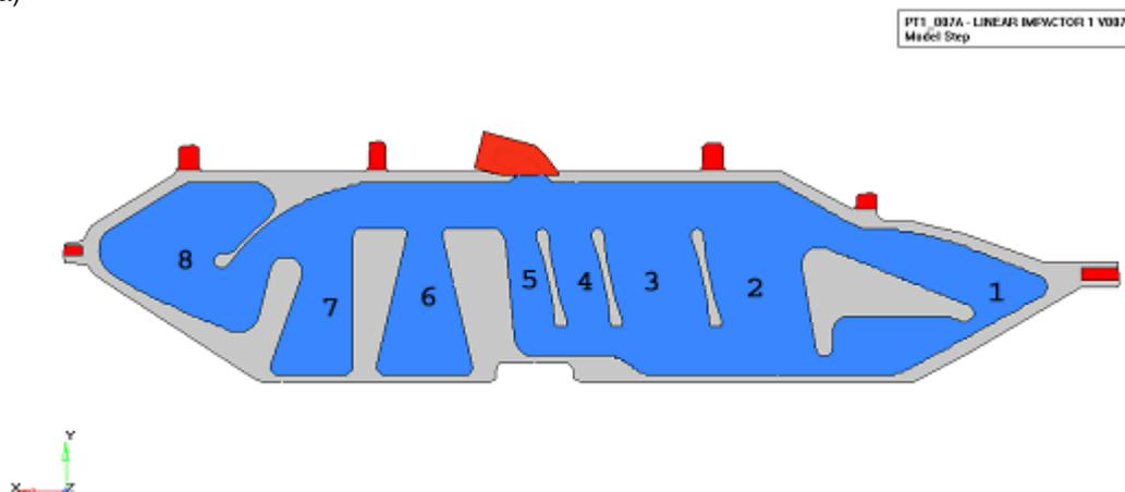
Figure 1: a) Curtain airbag. Blue- airbag chambers 1-8, grey – connecting fabric, red – fixation.
