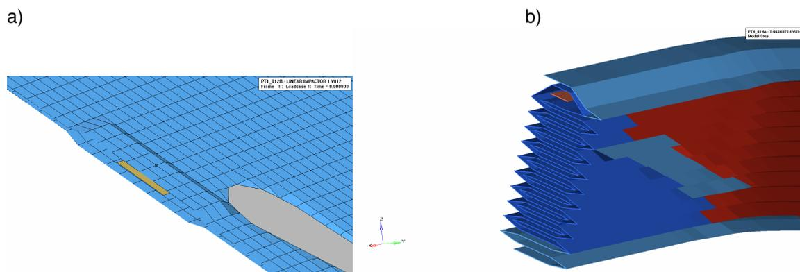
Figure 5: Gas generator model for unfolded airbag a) and folded airbag b). Airbag layer are moved from each other to let several ALE cells between
