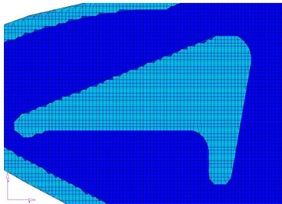
Figure 2: Mesh on the window airbag meshed. Dark blue- airbag chambers, light blue – connecting fabric.
