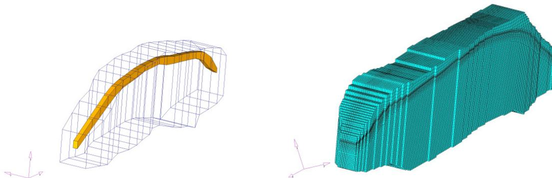
Figure 4: Airbag envelope space (blue wire frame lines) and initial position of the folded airbag (yellow box). Corresponding ALE mesh is denser near the initial position of the folded airbag. Mesh fills only the airbag envelope space. ALE mesh size is approx. 300.000 cells
