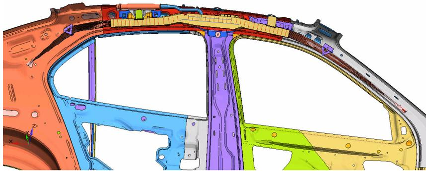
Figure 4: Curtain airbag after bending is integrated into the actual body-in-white surrounding
