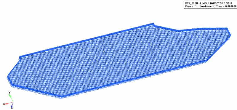
Figure 5: ALE mesh for a push-up test. Increased mesh density towards the flat table. ALE mesh with approx. 150.000 cells
