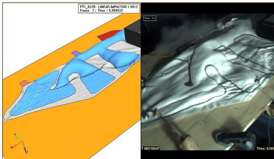
Figure 6: Push- up test after 6ms. Impactor to the driver compartment.
