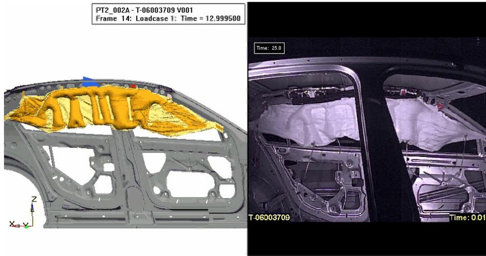
Figure 8: Blow up test. Comparison simulation and test after 13ms
