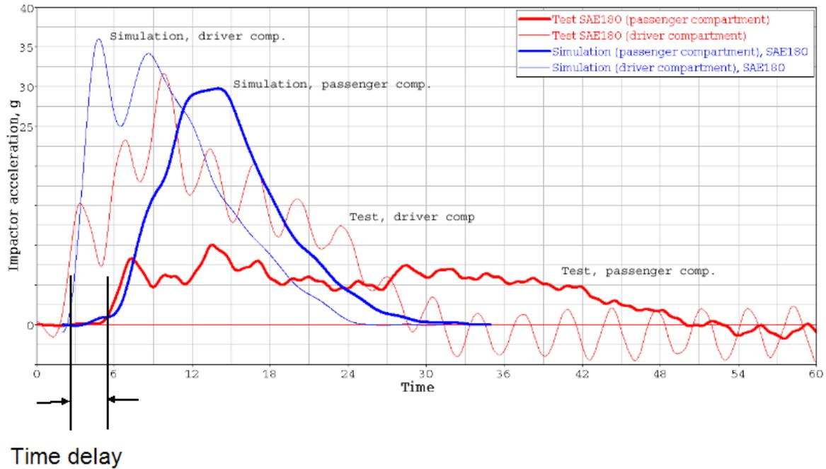
Figure 7: Push-up test. Comparison of the impactor accelerations. Impactor to the driver compartment (thin curves), impactor to the passenger compartment (thick curves)
