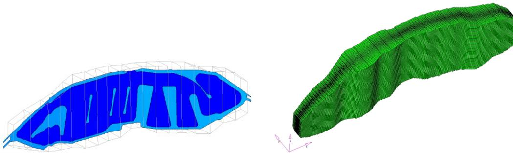
Figure 6: ALE mesh for a bended curtain airbag (not folded) in window opening. Denser mesh follows the initial position of the airbag. Mesh fills the airbag envelope space (grey wire frame lines). ALE mesh with approx. 250.000 cells
