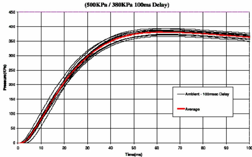
Figure 4: Gas tank pressure curve at ambient temperature and 100 ms delay (Source: Airbag manufacturer)
