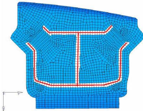
Figure 8: FE Airbag cover model (plastic shells)
