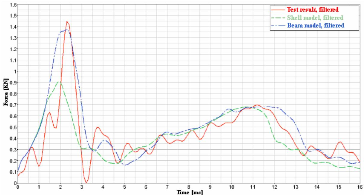
Figure 11: Airbag cover FE model: Comparison shell / beam model to test
