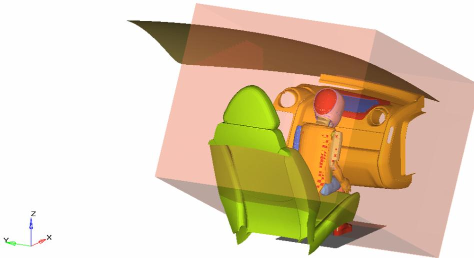
Figure 12: 3yrs dummy with head at cockpit, complete simulation model
