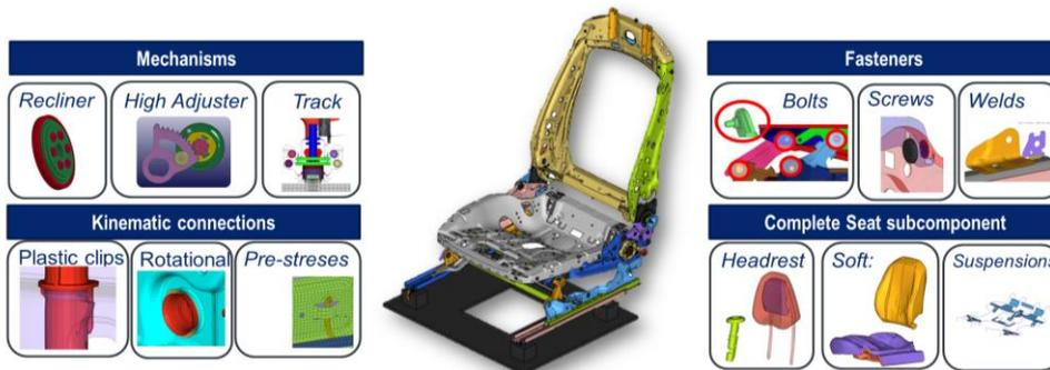
Fig.1: Typical connections for car seat.
