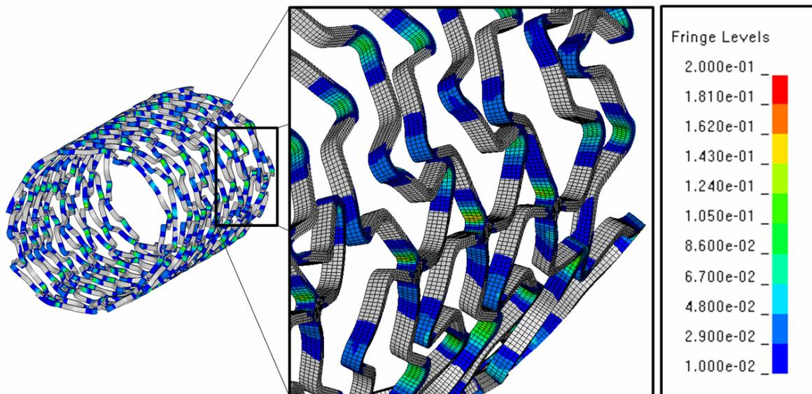
Figure 4-3: Fringe Plot of Failure Risk after Crimping, Dilatation and Recoil.
