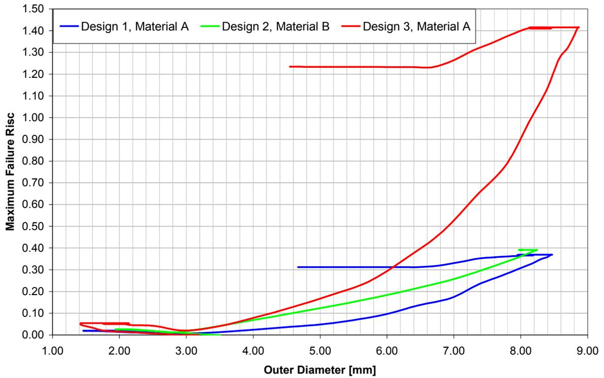
Figure 4-2: Maximum Failure Risk against outer Diameter.
