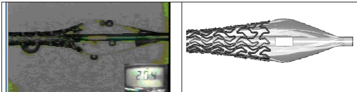
Figure 5-1: Qualitativ comparison of „dog bone" effect of in vitro (with courtesy of BSCI TZ GmbH) and simulation. Here different stent designs are depicted.
