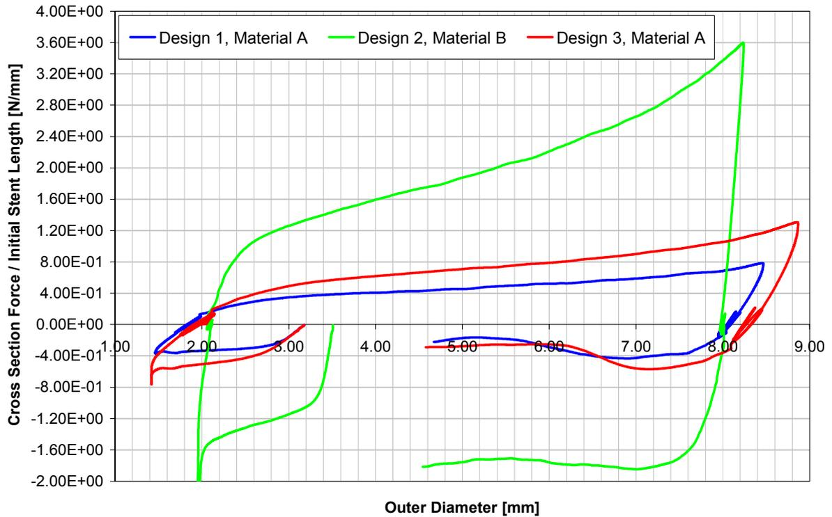
Figure 4-1: Cross Section Force against outer Diameter.
