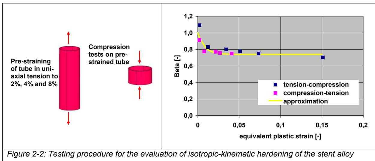
In order to test the isotropic-kinematic hardening model of material model MF-GenYld one hexagonal solid element is used in to simulate tension-compression reversal tests with different levels of pre-strain in tension. Figure 2-3 gives the resulting stress-strain curves which clearly indicate the Bauschinger effect. Additionally the evolution of the parameter  $\beta$  as a function of prestraining is shown
