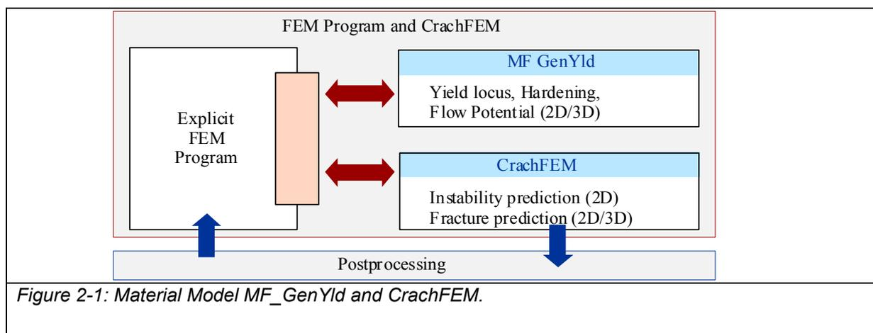
The models in CrachFEM for the prediction of material failure due to shear fracture and ductile fracture in metallic materials (these criteria are used for solid elements) are discussed and compared with other types of fracture models in [2] and not reported here.
