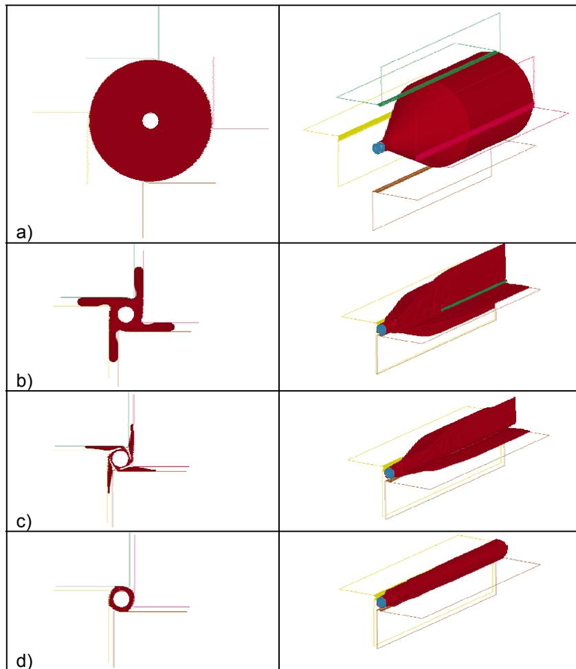
Figure 1-1: Simulation of balloon folding process
