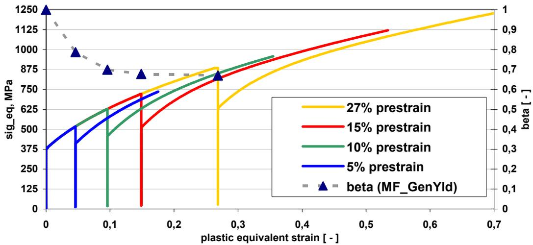
Figure 2-3: Stress versus plastic strain from simulation of tension-compression reversals with different pre-straining in tension with LS-DYNA user-material model MF\_GenYld.
