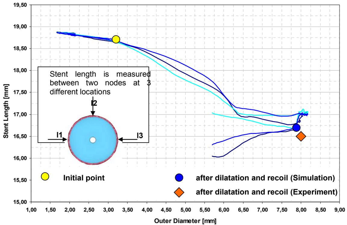
Figure 4-4: Stent length vs. outer diameter (Balloon dilatation).
