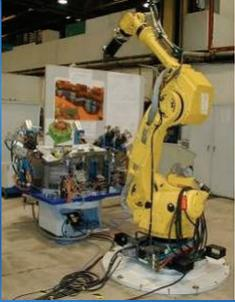
Complete system (robot and hemming fixture for 3305 Astra HB3)
