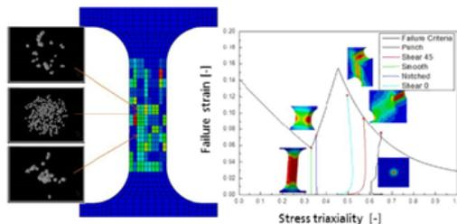
Mapping of local thickness, voids, derived damage from flow path length & Temp. or residual stresses
