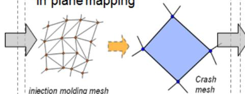
Mapping in thickness direction
