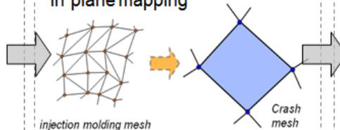
Mapping in thickness direction
