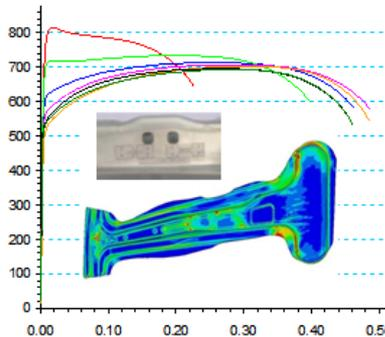
Mapping of local properties like thickness, pl. strain, damage or stresses
