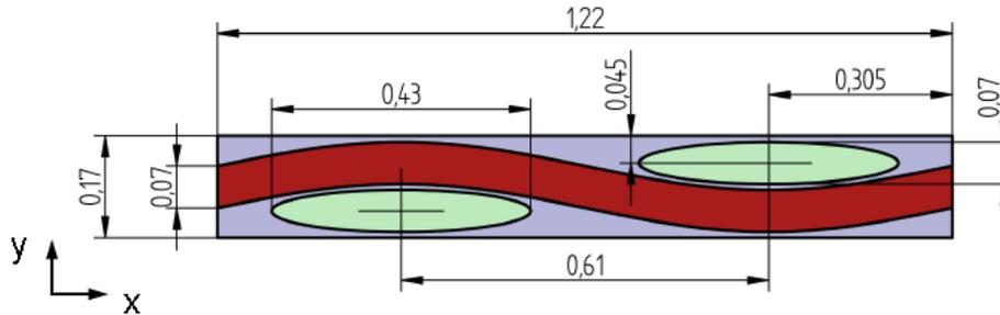
Fig. 3: Exemplarily selected cross section for a representative sequence according to MATSUDA et. al [4] used for the investigations in the Finite-Element-Analyses: Warp yarn (red), Weft yarn (green), matrix (blue).
