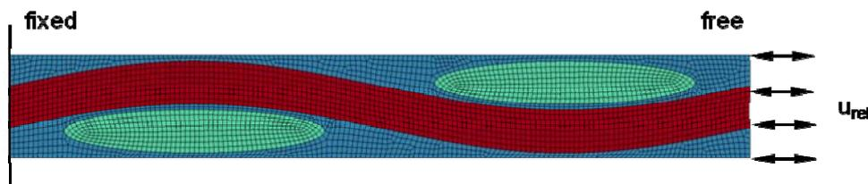
Fig. 4: Modeled cross section, discretization and boundary conditions for the selected representative sequence according to MATSUDA et. al [4] used for the investigations by the FE-Analyses.
