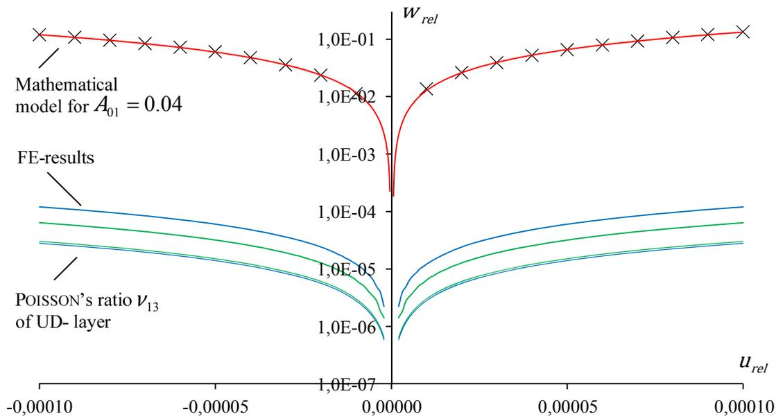
Fig. 6: Single-logarithmically scaled  $w_{rel} - u_{rel}$ -diagram obtained for the different investigations: Red solid line: Mathematical model; Upper blue solid line: FE-results for carbon fiber; Upper green solid line: FE-results for basalt fiber; Lower blue solid line: Amount of POISSON's ratio for carbon fiber; Lower green solid line: Amount of POISSON's ratio for basalt fiber.
