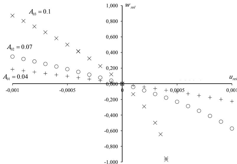
Fig. 2: Relative shift of the amplitude  $w_{rel}$  against the applied respective degree of deformation  $u_{rel} = -0,001 \dots +0,001$  for the selected amplitudes  $A_{01} = 0.04$ ,  $A_{02} = 0.07$  and  $A_{03} = 0.1$ .
