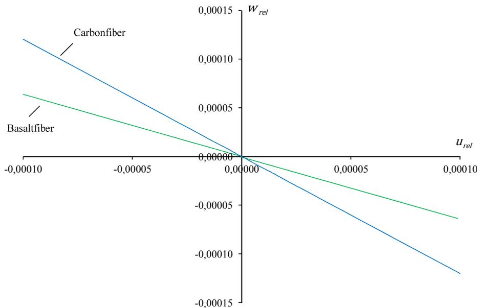
Fig. 5:  $w_{rel} - u_{rel}$ -diagram obtained by different fiber reinforcements in the same matrix system: Blue: Carbon fiber; Green: Basalt fiber.
