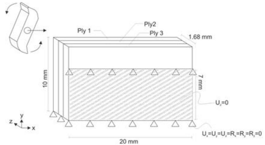
**Process:** Side milling (dry) with simplification of the workpiece thickness \* $t = 1.68$  mm
