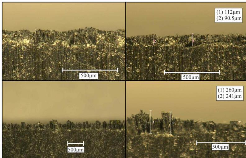
Visible surface delamination but no delamination between the plies detected
