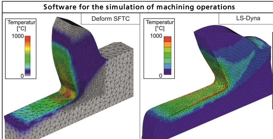
Approximation and close analysis of the high thermo-mechanical loading conditions inside the process
