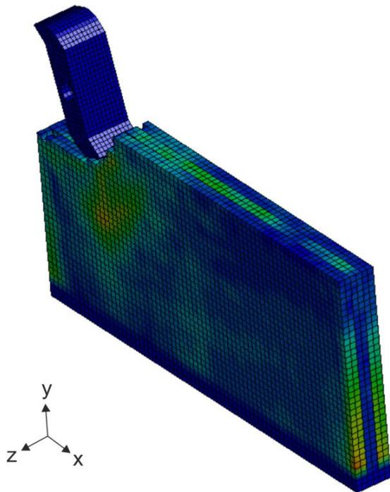
Work piece: 3 Layers of UD-CFRP (90°/0°/90°)
