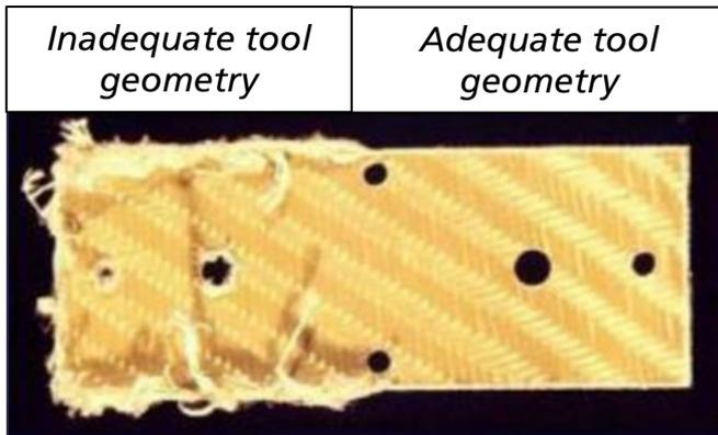
Visible fiber linting (left side) after machining an aramid fiber composite with an inadequate tool geometry
