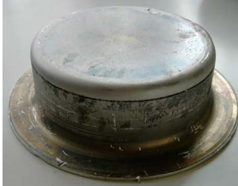
Figure 5: Experimental Result of a warm formed sheet metal aluminium alloy
