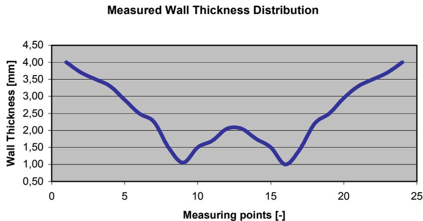
Figure 6: Diagram showing the absolute values of the measured wall thickness distribution of a formed part
