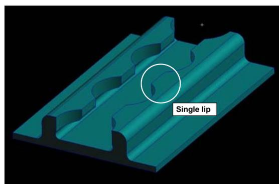
**Fig. 13:** Section of an aircraft floor rail for seat attachment
