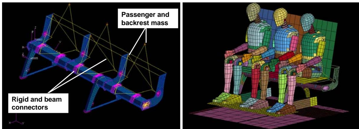
Fig. 11: AECS finite element model: MSC Nastran (left) and LS-Dyna (right)
