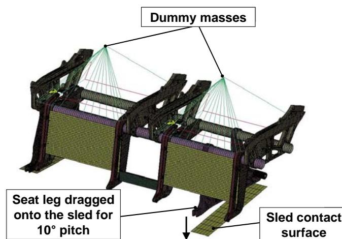
Fig. 21: Pre-deformation of the BC seat
