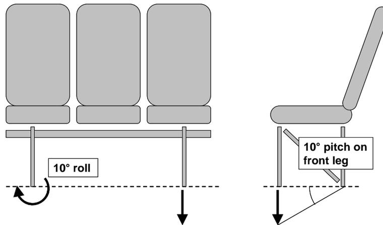
**Fig. 8:** Pre-deformation applied for structural test
