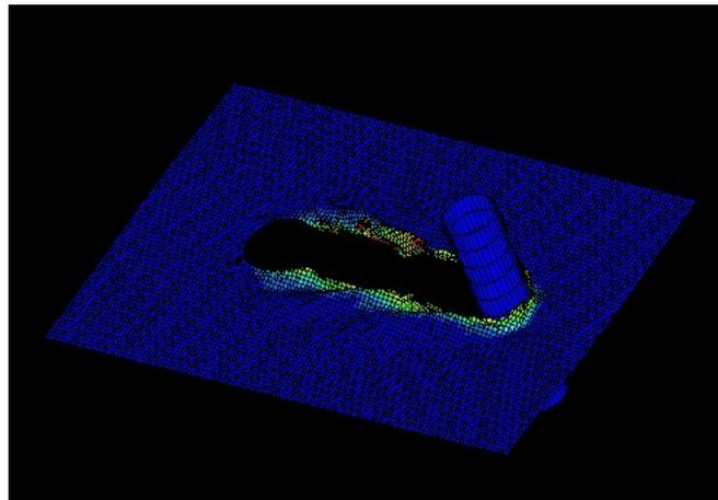
**Fig. 20:** Rigid bolt pulled through a laminated composite plate
