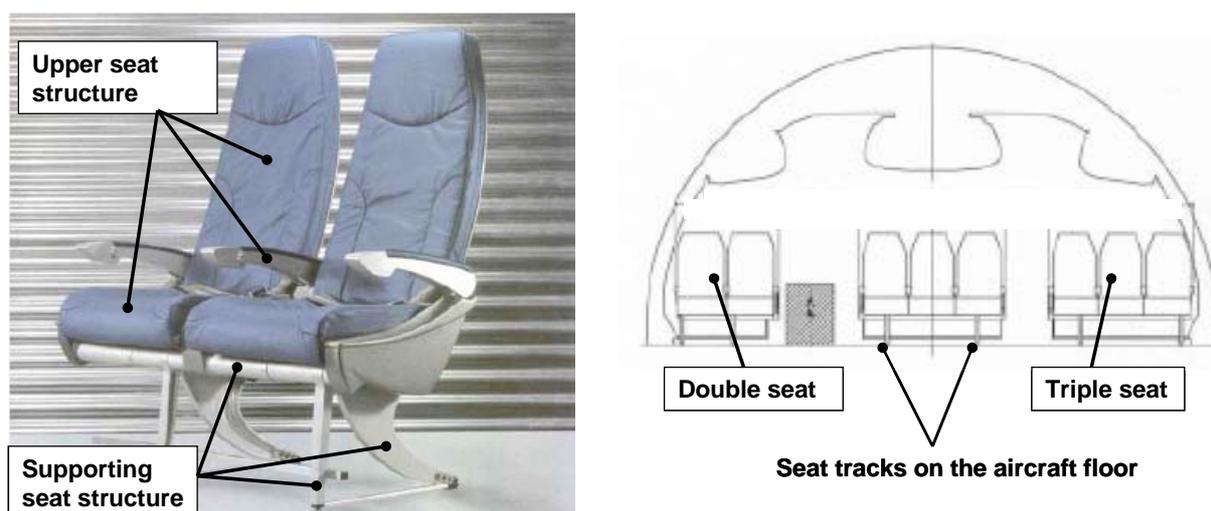
**Fig. 1:** Double seat configuration (left) and seat layout of an Airbus A340 aircraft
