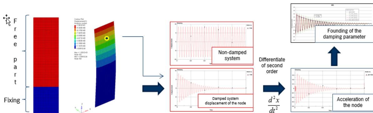
Fig. 1: Analytical reverse analysis and figure of the damping coefficient verification in LS-DYNA
