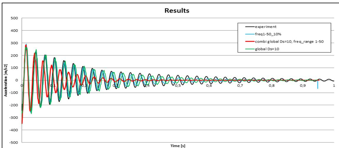
Fig.9: The comparison analysis of the \*DFR, \*DG and combination of both setups together
