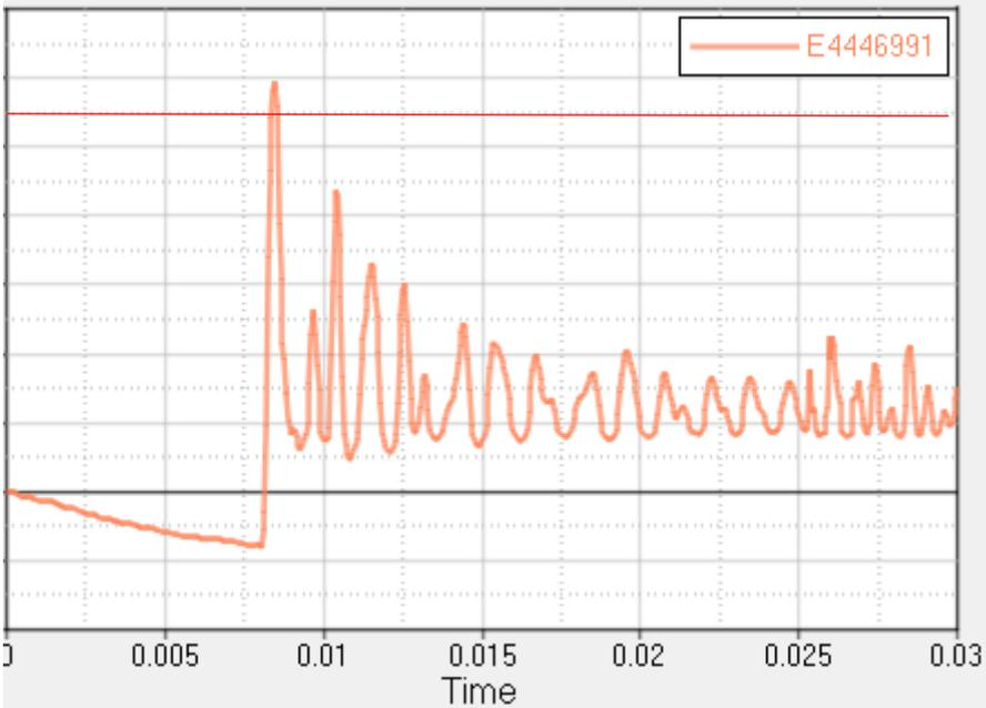
Fig. 17: Stress oscilation without damping
