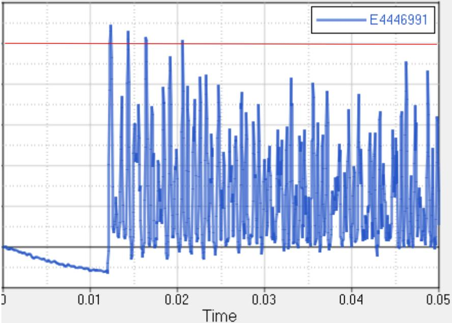
Fig. 16 Stress oscilation without damping
