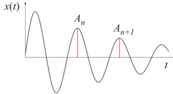
Fig.2: Scheme of the of the amplitudes for underdamped system - oscillator
