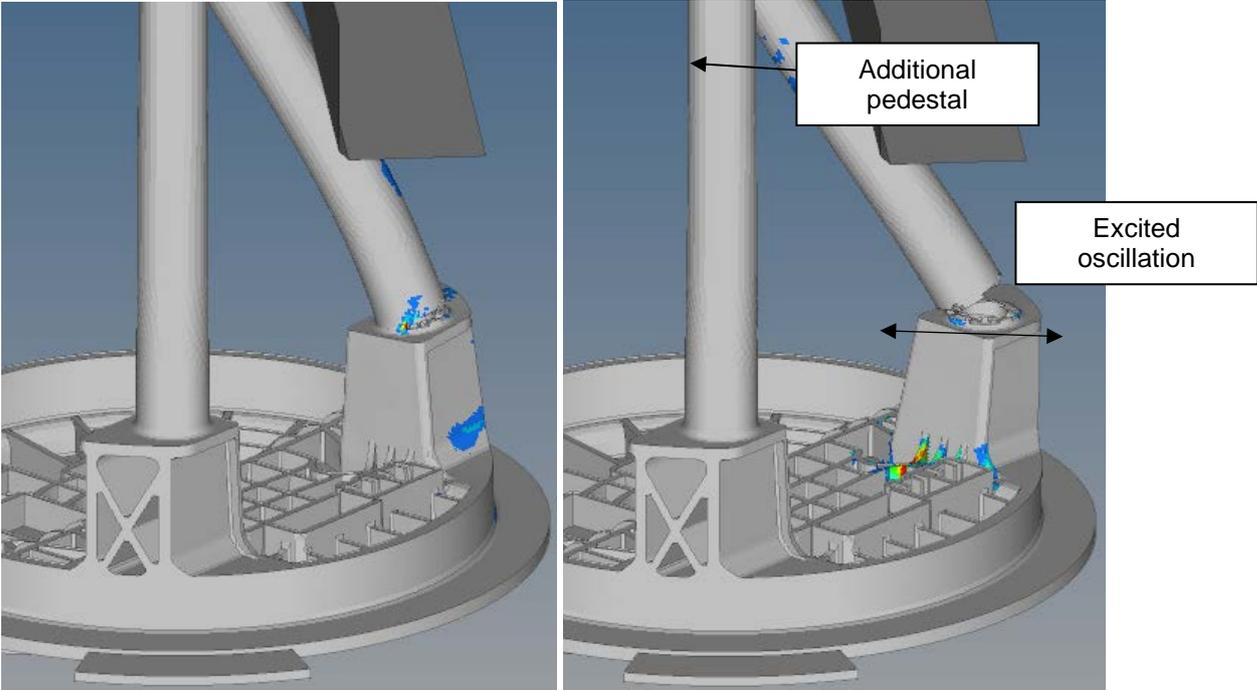
*Fig. 15: Impact test simulation of prolonged guiding rods*
