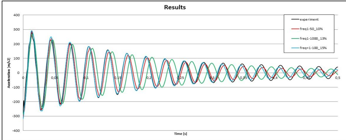
Fig.6: Different setup of the \*DAMPING\_FREQUENCY\_RANGE (\*DFR) and percentage elasticity change
