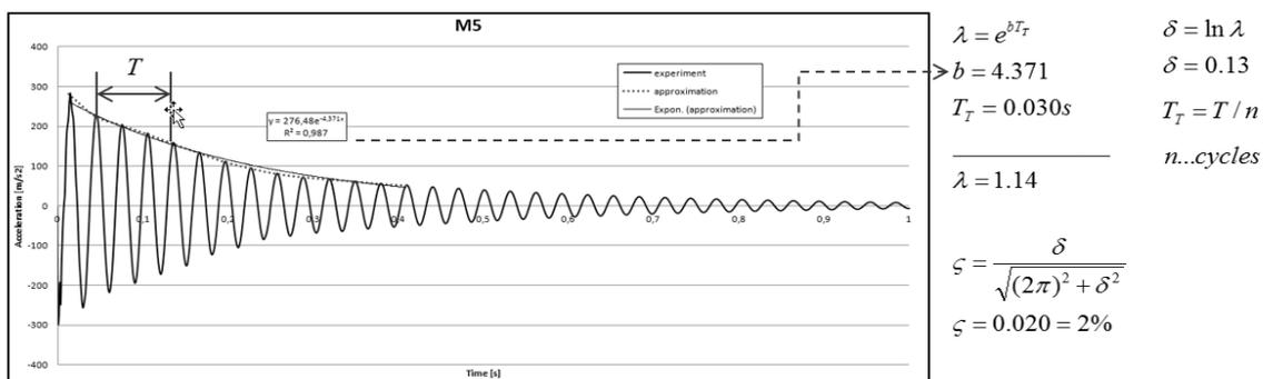
Fig.3: The determination process of the damping ratio from logarithmic decrement
