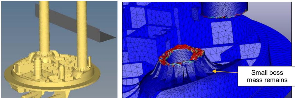
*Fig.12: Simulation of Bosch Impact Test (original design)*
