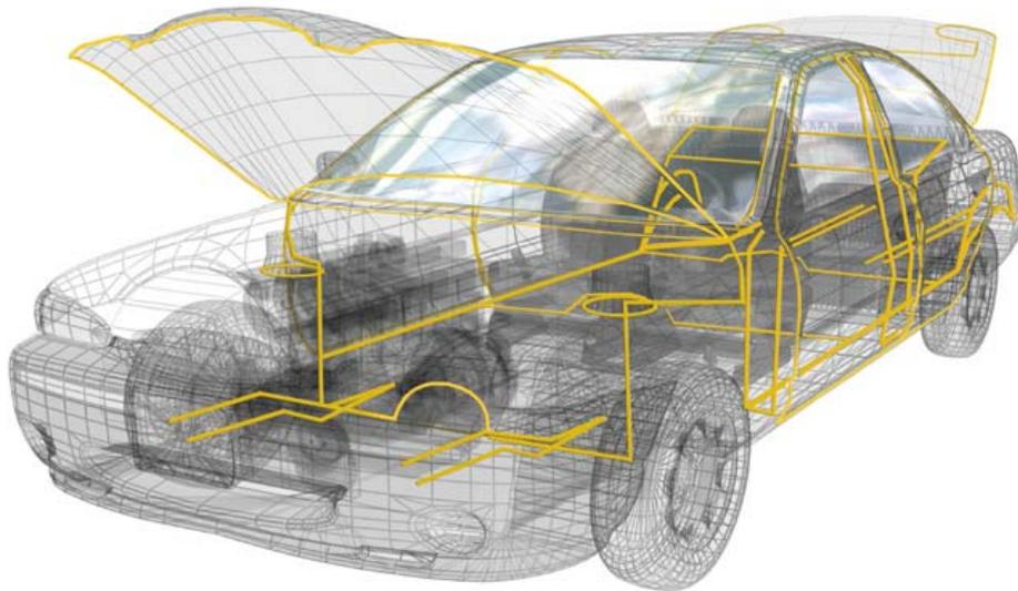
Figure 1: Potential structural adhesive bondline in the car body
