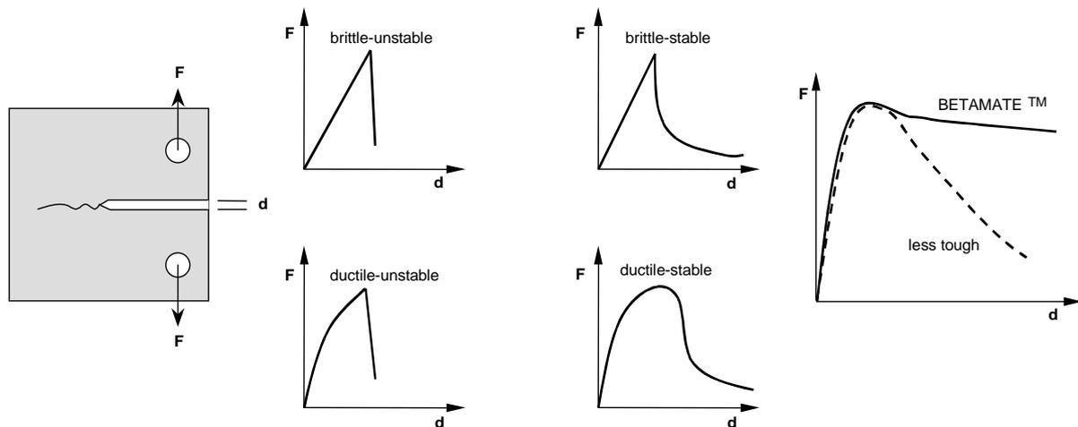
Figure 2: Adhesive CTS: crack initiation and propagation of different adhesive types
