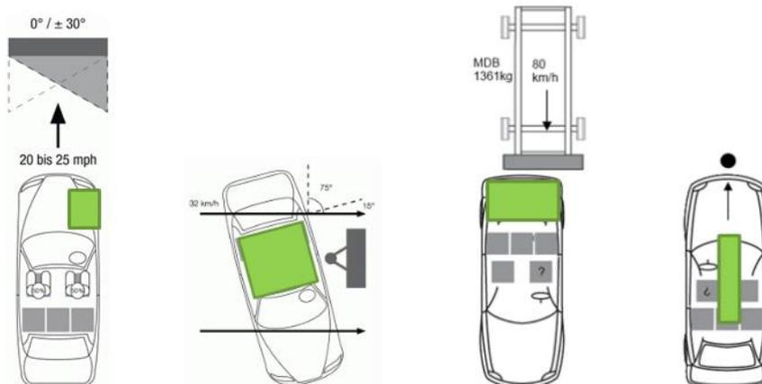
Fig.19: Results about the most critical scenario might strongly differ depending on the battery placement (green).
