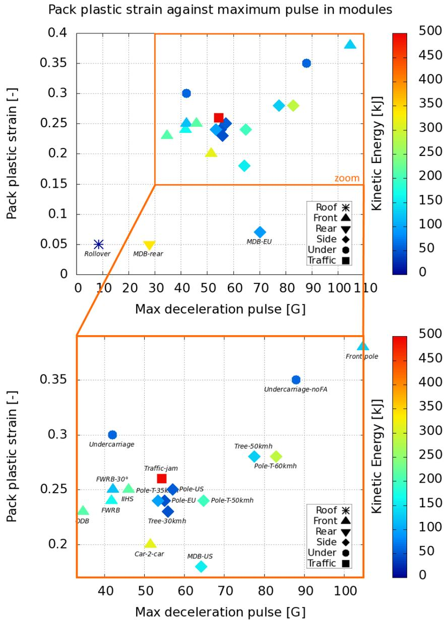
Fig.15: Simulation results in terms of battery pack plastic strain and maximum acceleration recorded in the modules, comparison between the different scenarios. The initial kinetic energy involved in each load case is also represented.
