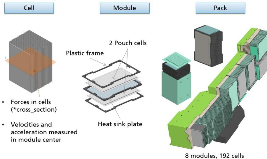
Fig.4: Battery pack model developed.
