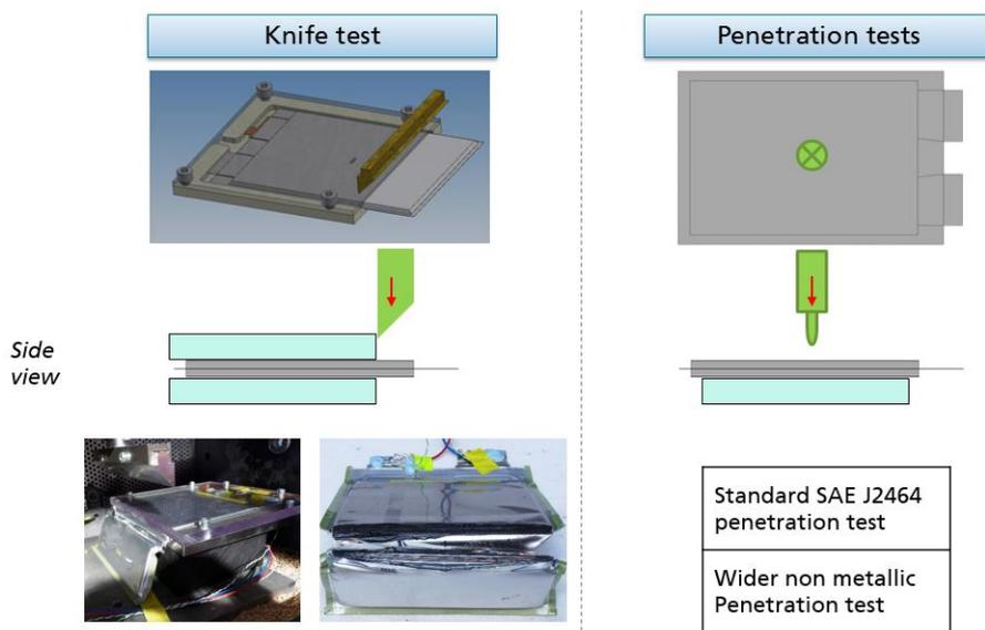
Fig.3: Mechanical abuse tests performed on Li-ion pouch cells: shear test with a knife (left) and penetrations tests according to standard and in-house test (right).
