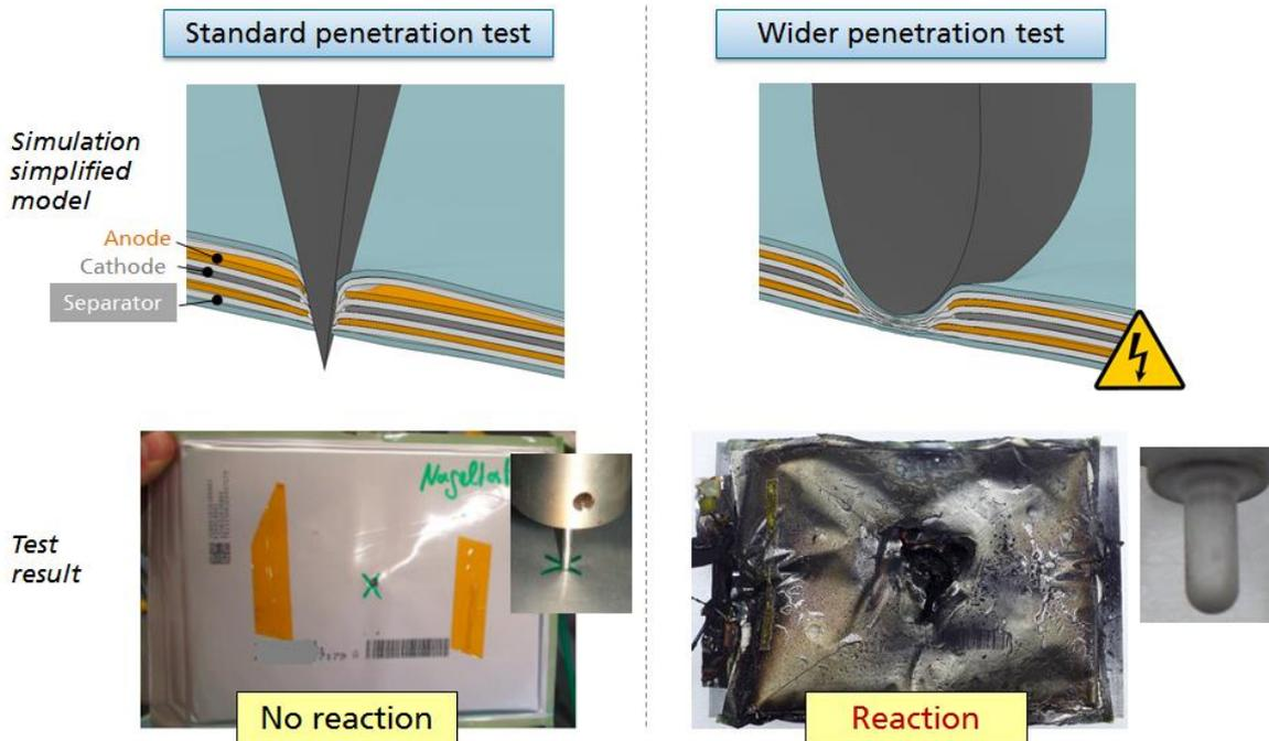
Fig.14: Differences in failure mechanism between standard penetration test (left) and wider penetrator (right), simplified simulation model.
