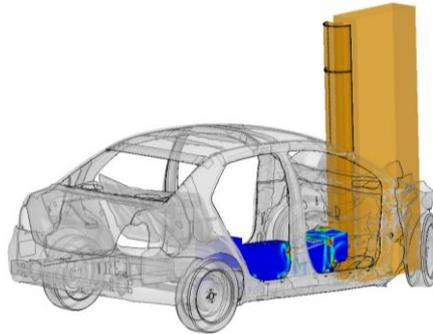
Fig.9: Front pole impact simulation for the 1GEV model developed within the project.
