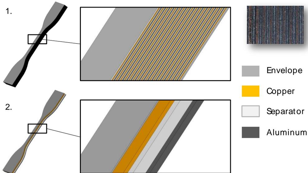
Fig.12: Numerical Model of Battery Cell (1-Detailed, 2-Simplified).
