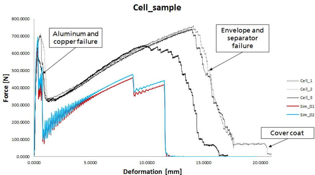
Fig.13: Validation of the cell model.
