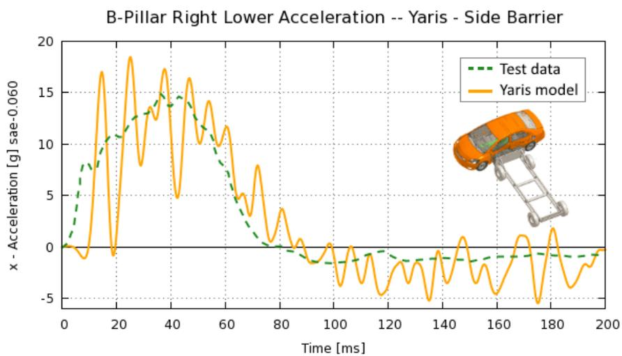
Fig.6: Crash pulses of Euro NCAP side barrier simulation for Toyota Yaris model. The orange curve denotes the numerical results; the green curve denotes test data of small family class vehicles.
