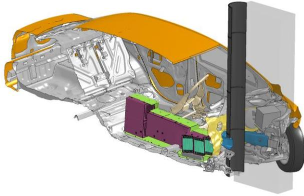
Fig.17: Front pole impact with 50 km/h. This scenario was found to be the most severe for the battery in terms of maximum forces in cells and maximum accelerations in the modules.
