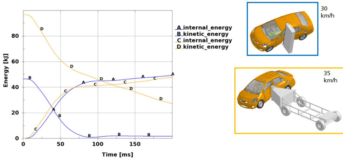
Fig.11: Very similar amount of deformation energy between Euro NCAP Side Pole (A curve) and reverse test performed (C curve).
