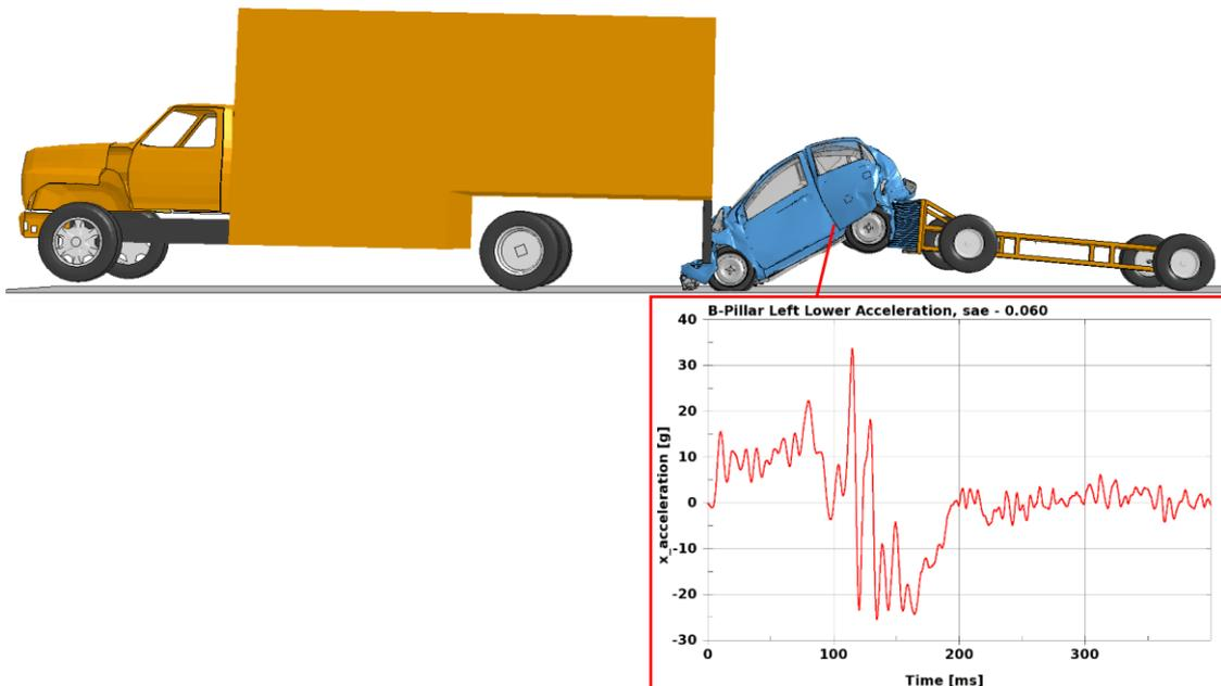
Fig.18: Simulation of a traffic jam accident.
