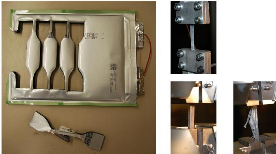
Fig.2: Tensile tests performed on pouch cells and on each layers.
