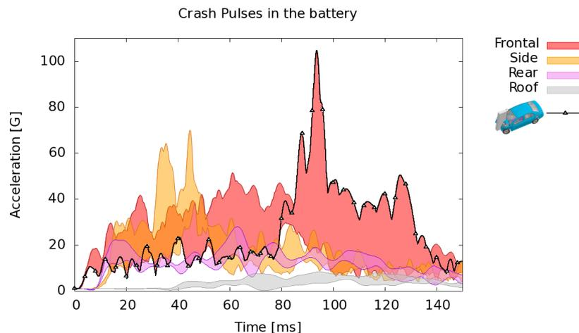
Fig.16: Acceleration corridors in the battery for frontal, side, rear and roof scenarios. Worst case scenario (front pole impact) is represented.
