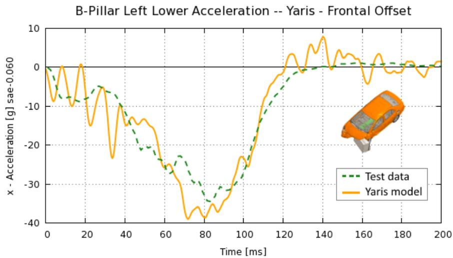
Fig.5: Crash pulse of Euro NCAP frontal offset simulation for Toyota Yaris model. Measurement is performed in the B-pillar. The orange curve denotes the numerical results; the green curve denotes test data of small family class vehicles.
