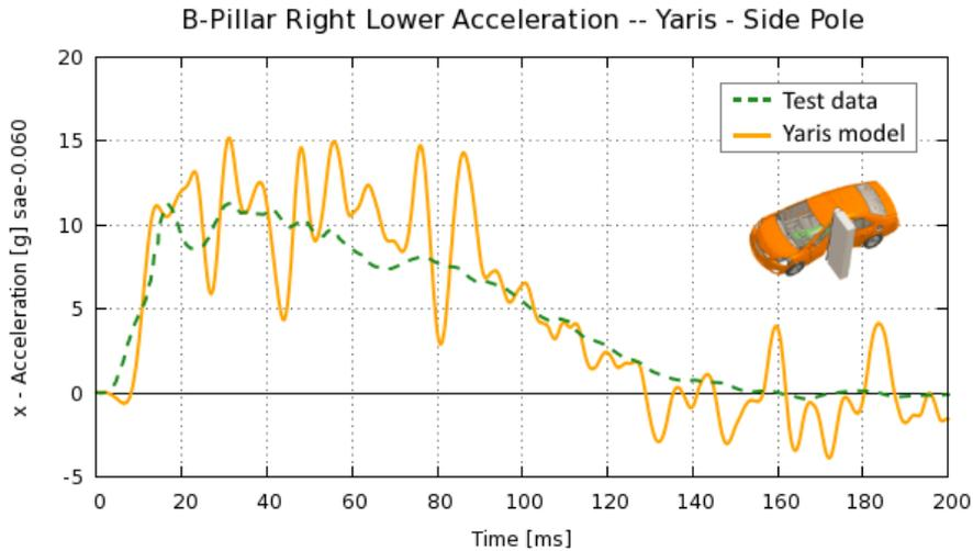
Fig.7: Crash pulse of Euro NCAP side pole simulation for Toyota Yaris model. The orange curve denotes the numerical results; the green curve denotes test data of small family class vehicles.
