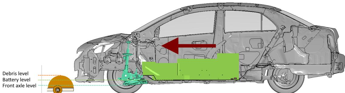
Fig.10: Undercarriage impact simulation, level differences between debris, battery and front axle.
