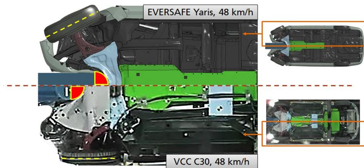
Fig.20: Comparison in front pole impact between VCC C30 at 48 km/h (bottom) and Toyota Yaris 1GEV at the same velocity (top).
