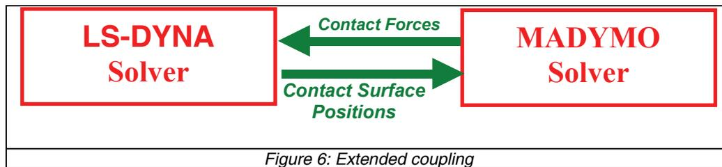
Figure 6: Extended coupling
