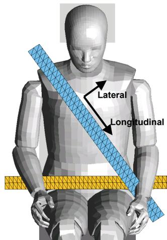
Figure 3: Facet dummy with FE belt
