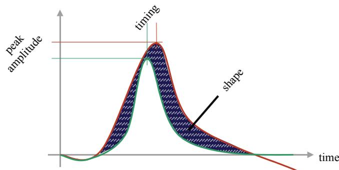
Figure 4: Three different criteria used for signal comparison.
