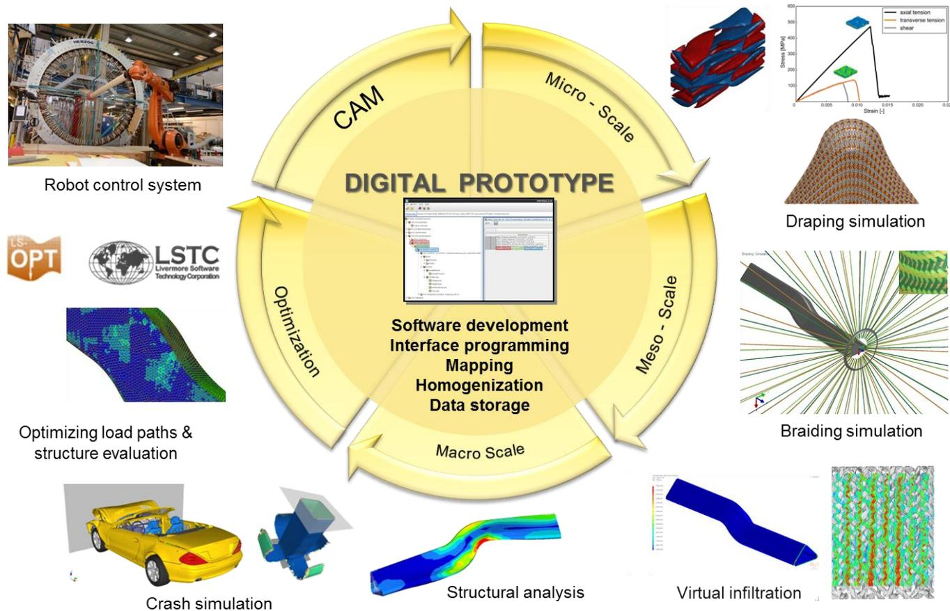
**DigitPro – the Digital Prototype: closing the simulation process chain**
