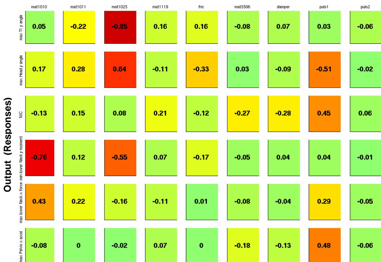
Figure 27: Correlation matrix displays significance of input parameters with respect to output values
