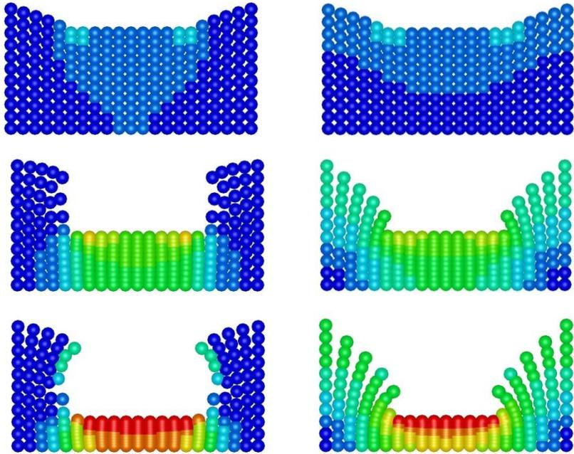
Punch test with (left) and without **tensile instability** (right)
