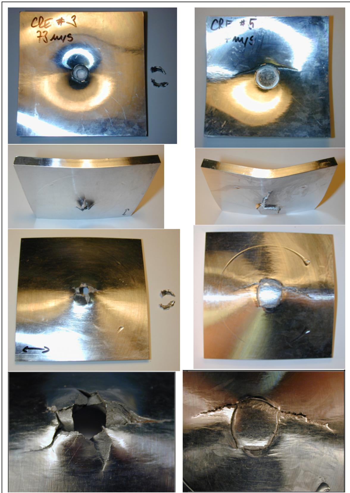
Figure 20: Critical damage patterns
