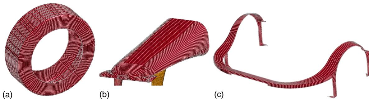
Fig. 2: Unstructured mesh after batch meshing, (a) wheel, (b) nose of a sports car, (c) bumper. White lines show basic material orientation.
