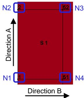
Fig. 3: Material axes determined by element nodes N1, N2, and N4
