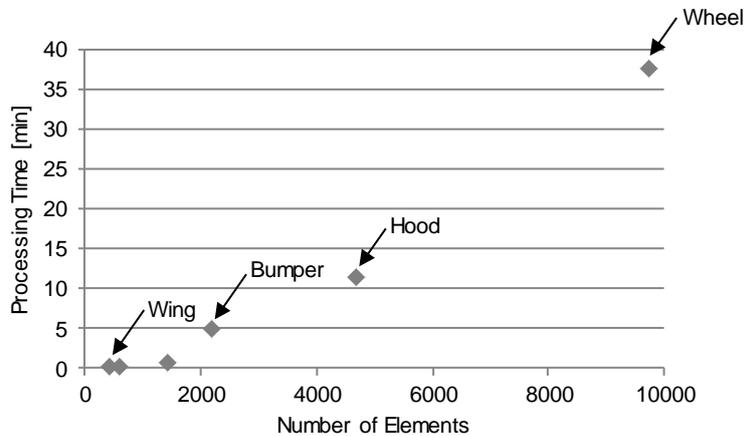
Fig. 8: Processing time of and number of elements of different example parts
