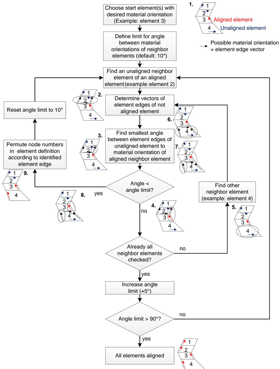
Fig. 4: Operating principle of the aligning algorithm
