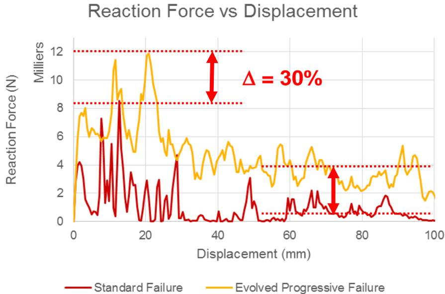
Post failure behavior of progressive failure model shows a higher residual stiffness
