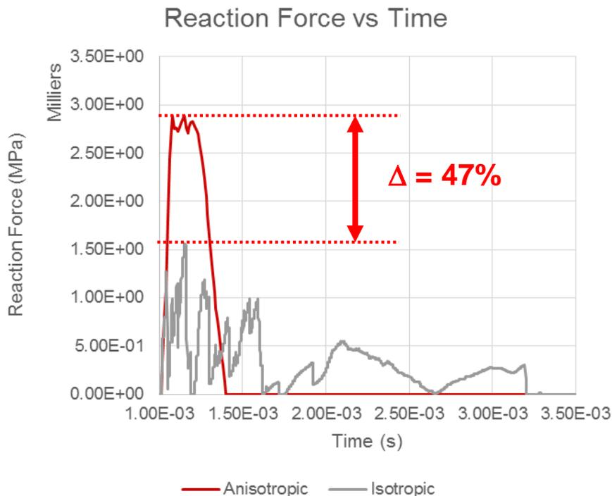
The anisotropic material model shows a much highest capacity of energy absorption during the impact.
