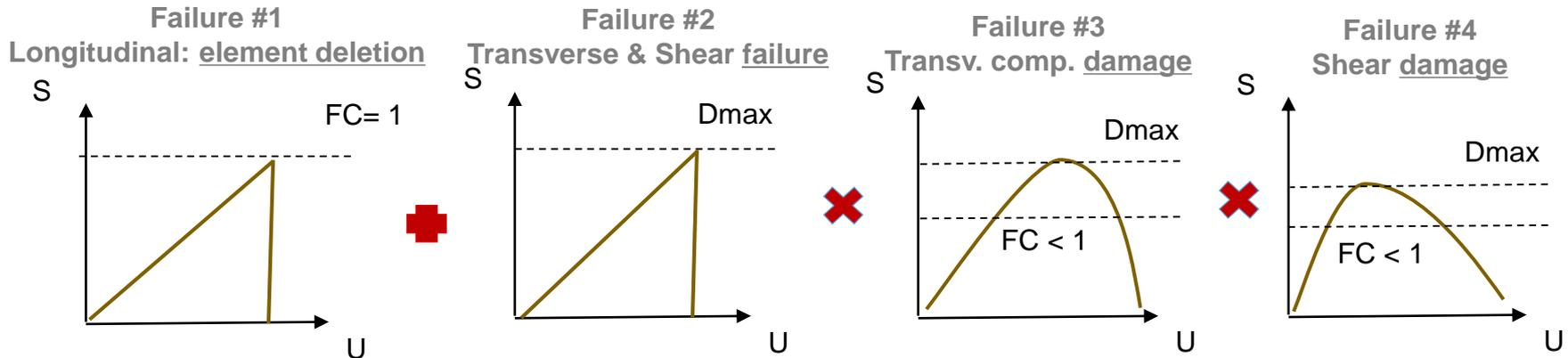
**Evolved progressive failure → anisotropic definition of the damage evolution with crack propagation**
