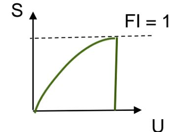
**Element deletion → brutal loss of stiffness in all directions**
