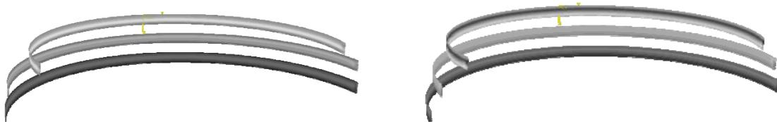
Fig.5: Ring splitting simulation. Left: the current model, right: combined hardening ansatz.
