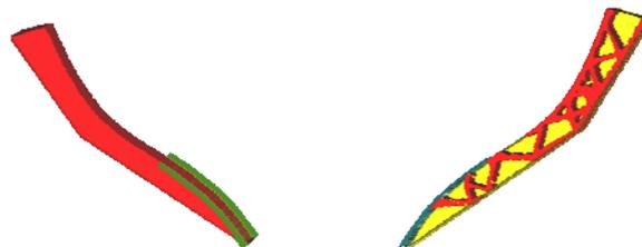
Figure 7. Topology Optimization. Initial and Final Designs
