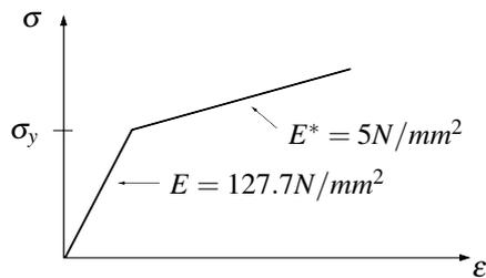
Figure 9: Stress-strain-curve
