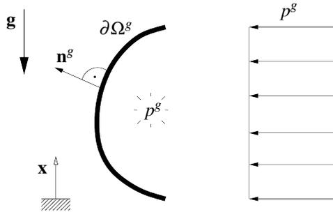
Figure 4: Pressure in a gas filled chamber
