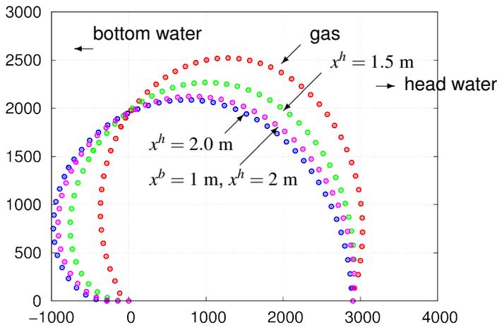
Figure 13: Red: Dam filled with gas ( $p = 0.0125 \text{ N/mm}^2$ ), Green: additional head water ( $x^h = 1.5 \text{ m}$ ), Blue: additional head water ( $x^h = 2 \text{ m}$ ), Pink: additional head and bottom water ( $x^b = 1 \text{ m}, x^h = 2 \text{ m}$ )
