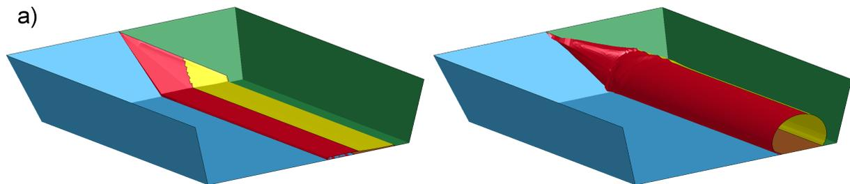
Figure 10: Model: a) initial state of uninflated tube and b) final state of the inflation with gas
