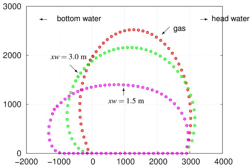
Figure 12: Cross-section deformation for different fillings
