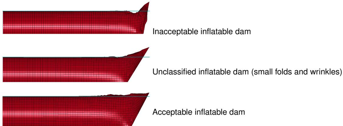
Figure 2: Influence of geometric parameter variation on folds and wrinkles
