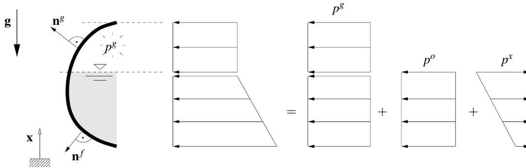
Figure 6: Hydrostatic pressure of a fluid and gas filled chamber
