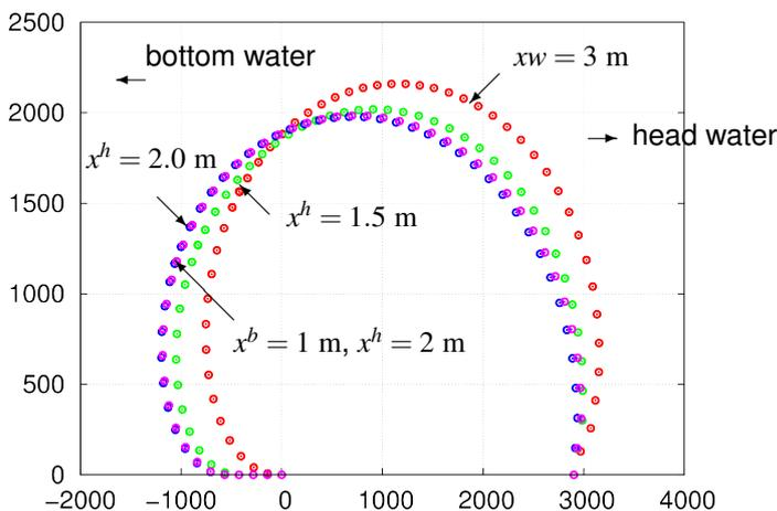
Figure 14: Red: Dam filled with fluid ( $x_w = 3 \text{ m}$ ), Green: additional head water ( $x^h = 1.5 \text{ m}$ ), Blue: additional head water ( $x^h = 2 \text{ m}$ ), Pink: additional head and bottom water ( $x^b = 1 \text{ m}, x^h = 2 \text{ m}$ )
