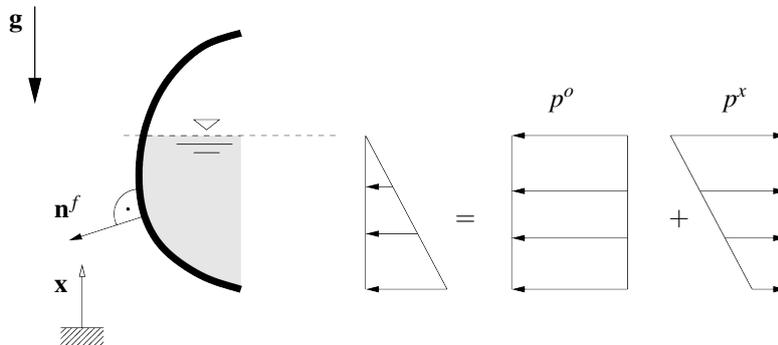
Figure 5: Hydrostatic pressure in a partially filled chamber
