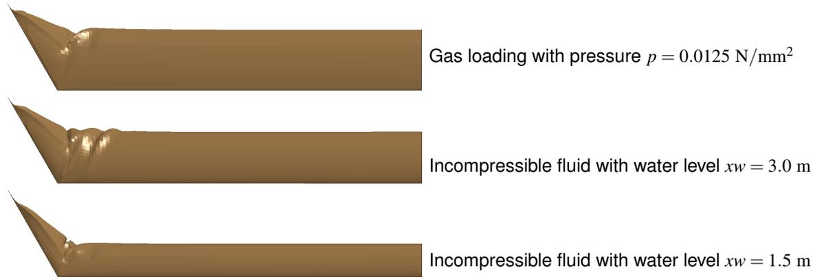
Figure 11: Filled inflatable dams with different media and different internal water height
