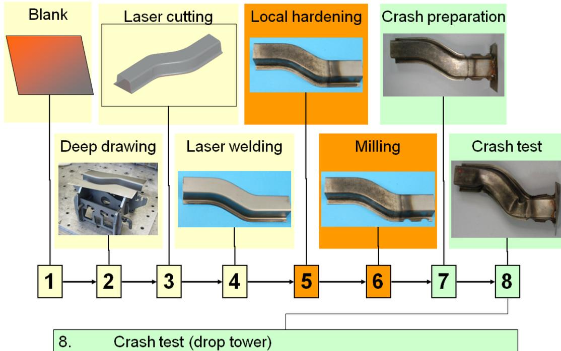
Figure 2: Manufacturing process from undeformed multi-phase steel sheet to locally hardened side rail in experimental crash test.
