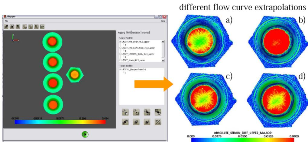
Figure 7: Different simulation results (LS-Dyna) mapped and compared to one experimental result (ARGUS)
