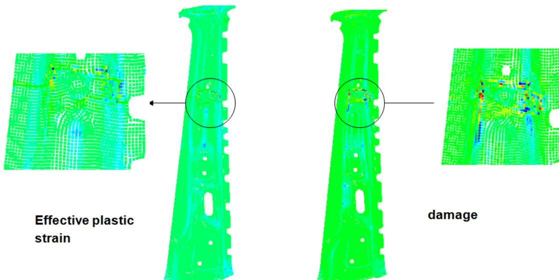
Figure 4: Differences of crash simulation with and without mapping at effective plastic strain and damage for a ZStE340 metal blank of a B-pillar.
