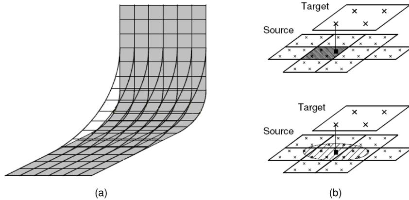
Figure 1: (a) Mapping between non-overlapping structures (b) Element section for the interpolation basis - modified Shepard algorithm [4] (bottom) in relation to element-based interpolation(top)
