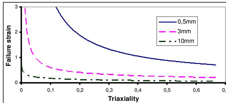
Figure 5: Failure curves for three element lengths of Aluminum material
