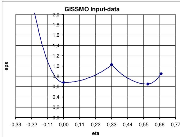
Fig. 1 GISSMO Input-data, failure strain versus triaxiality for plane stress
