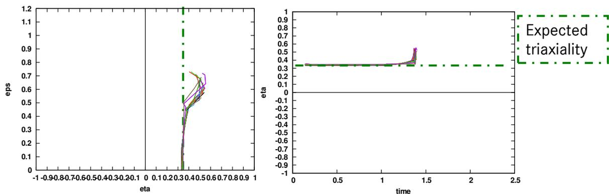
Fig. 10: Result of uniaxial tensile test; plastic strain vs. triaxiality and triaxiality vs. time
