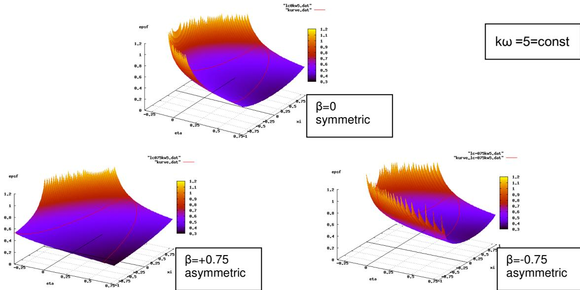
Fig. 4: Gurson – Hutchinson Failure surface, different values of  $\beta$
