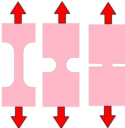
Fig. 8: tensile test specimens: Mini-MPA, FzR4, FzR1
