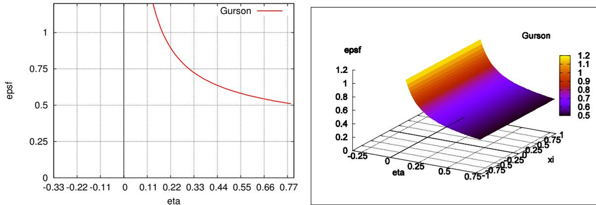
Fig. 2: Gurson model, failure curve and failure surface
