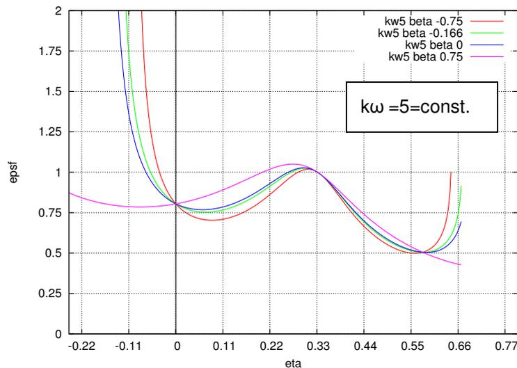
Fig. 6: Gurson-Hutchinson failure curve for different values of parameter  $\beta$
