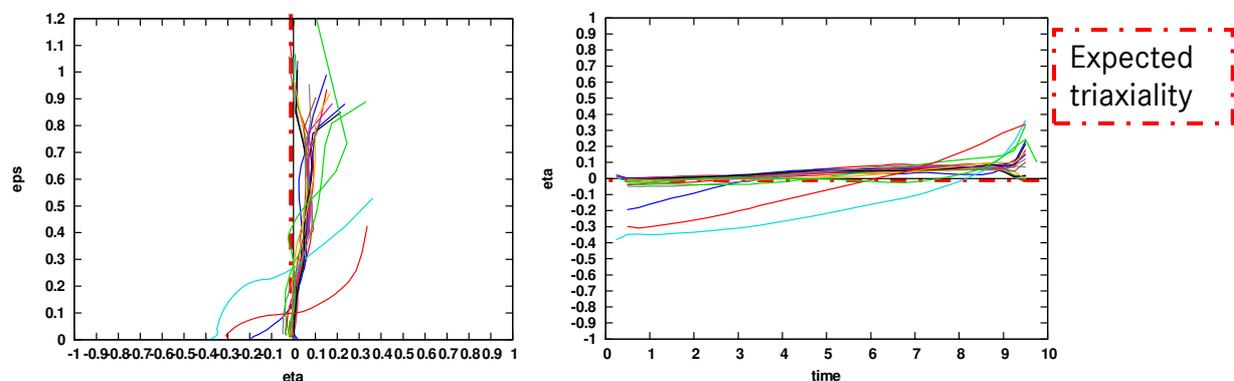
Fig. 11: Result of Iosipescu shear test; plastic strain vs. triaxiality and triaxiality vs. time
