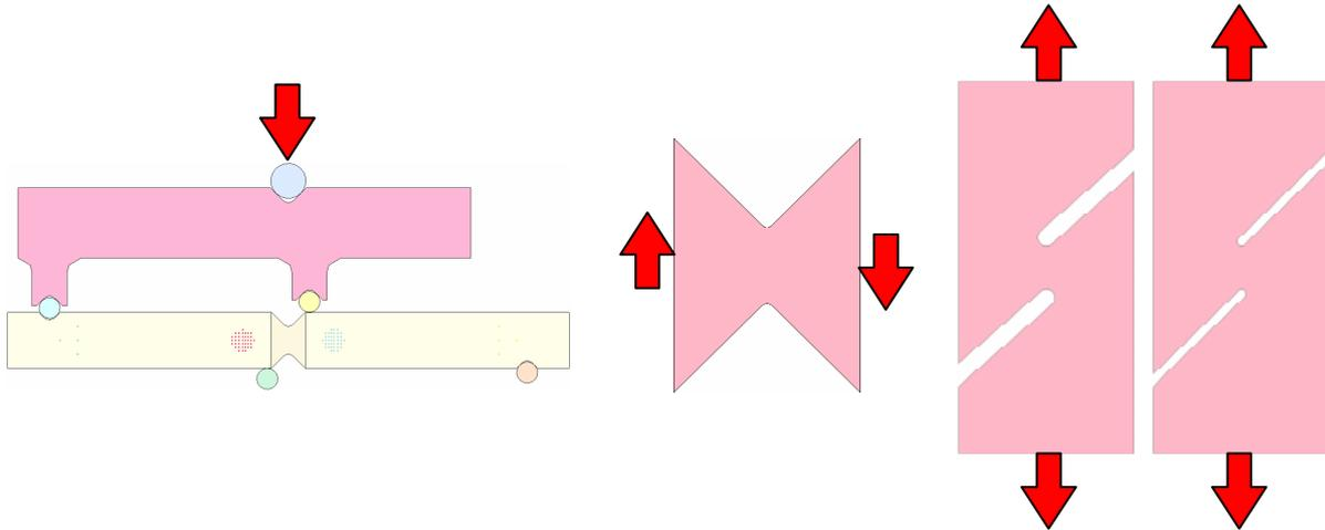
Fig. 7: Shear test specimens: Iosipescu, ARCAN, Scherzug R1 +R0.5
