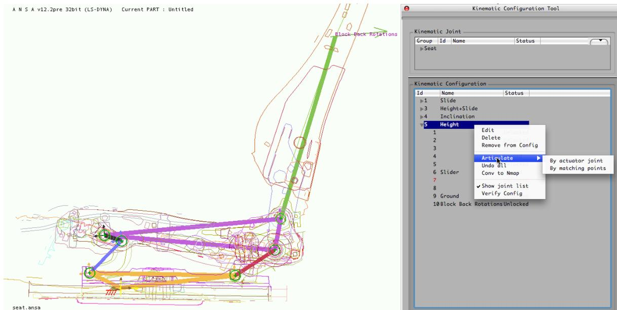
Fig. 2: A complete seat model with its various discrete movements predefined. (model courtesy of BMW)
