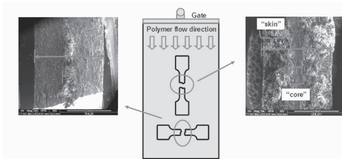
Fig. 2: Rupture surface of broken tensile specimen cut from plaque (SEM images, material: 40% GF PP homopolymer)
