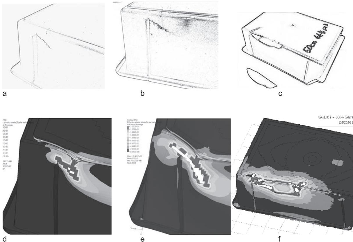
Fig.9: Box after the impact in the second drop test presented. Above: real test images, below virtual tests. From Left to right: SGF-Soft PP falling height 0.5 m, SGF-Soft PP falling height 0.8 m; 30 % SGF-PP falling height 0.5 m
