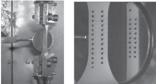
*Fig. 4: Experimental measurement of the  $r$ -values: a mirror is placed on a side of the specimen in the tensile test, in order to simultaneously measure the strain along its width and thickness using optical methods, based on the tracking of markers.*
